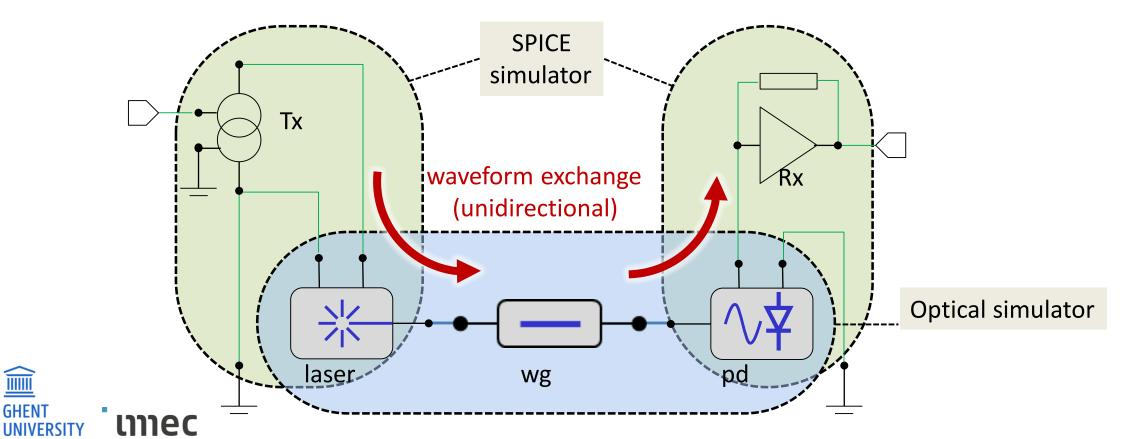
True cosimulation (photonics and electronics in lockstep)
