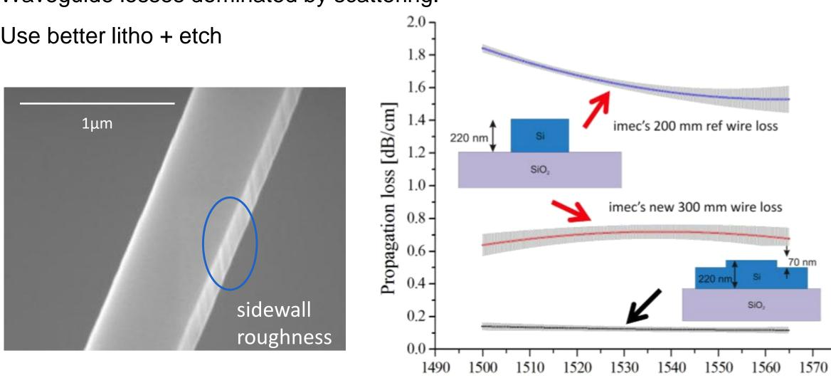
Waveguide losses dominated by scattering.
