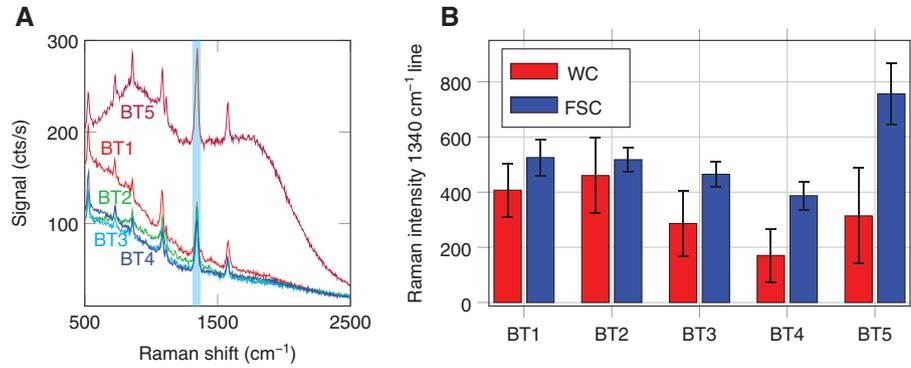
**Figure 4:** Free-space versus waveguide-excited single-antenna SERS spectra.
