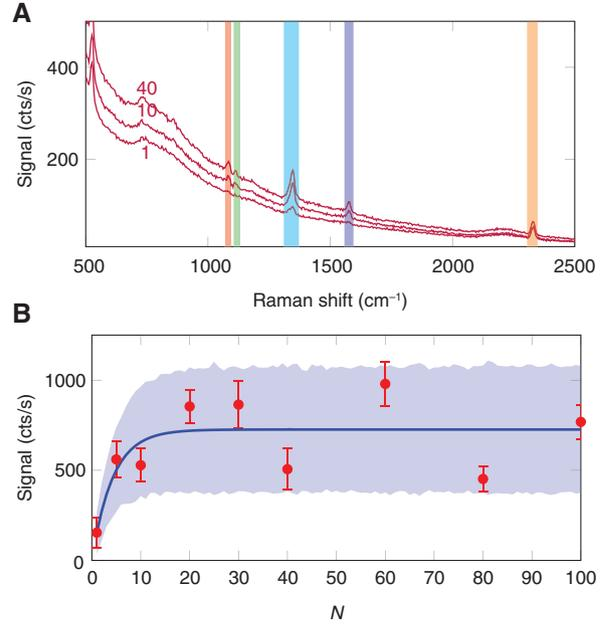
**Figure 2:** Waveguide-excited SERS signals for varying number of antennas.
