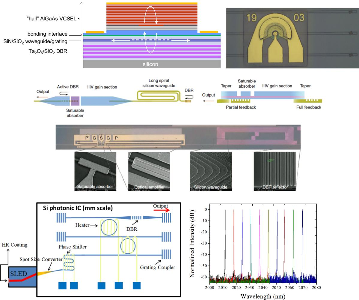
**Fig.1 Top:** Cross-section of the VCSIL showing the hybrid-vertical-cavity and the intra-cavity waveguide/grating for in-plane emission and microscope image of a VCSIL with the intra-cavity waveguide and one of the grating outcouplers visible. **Middle:** III-V-on-silicon modelocked lasers with 1 GHz repetition rate. **Bottom:** 2.  $\mu\text{m}$  GaSb/Si widely tunable laser with 60 nm tuning.
