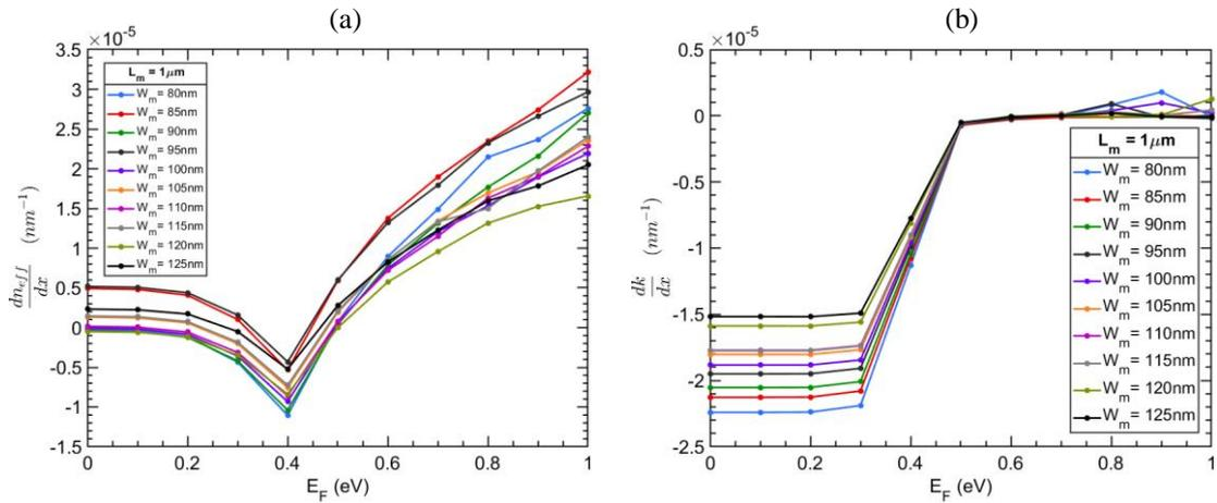
Fig. 5: Refractive index change per unit displacement of membrane as function of graphene fermi energy for different widths. (a) For real part of refractive index. (b) Imaginary part of refractive index.
