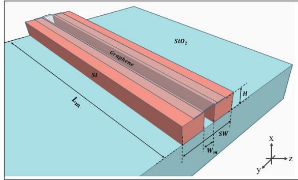
Fig. 1: Schematic of device under consideration: graphene (grey) is transferred onto a Si (brown) slot waveguide on oxide (blue). Parameters:  $SW = 500nm + W_m$  and  $H = 220nm$ .
