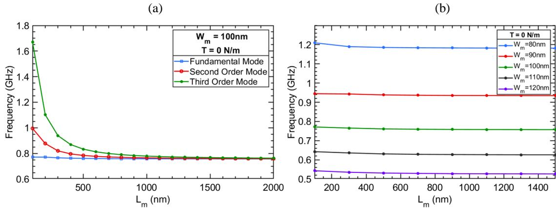
Fig. 2: Frequency vs membrane length. (a) For the first three modes under no tension. (b) Fundamental mode for different  $W_m$  under no tension. Note that the frequency becomes independent for  $L_m > 10 \times W_m$ .
