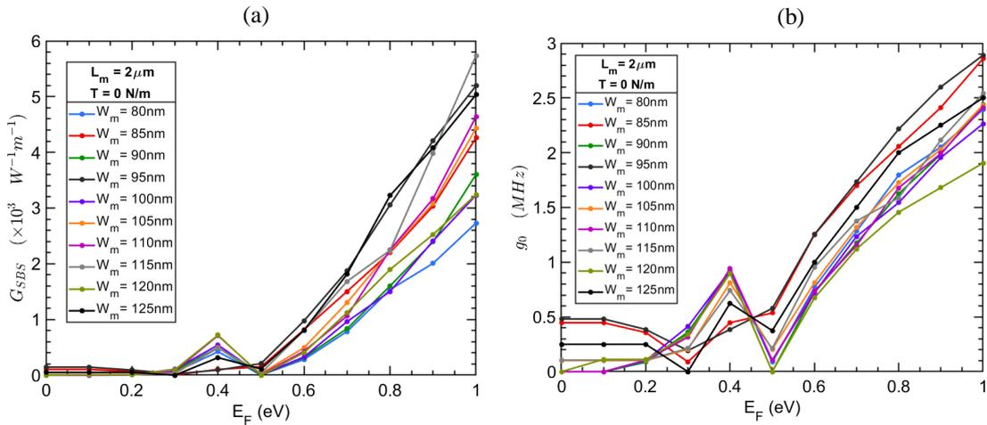
Fig. 6: Optomechanical figure of merits. (a) Brillouin gain vs graphene fermi energy for different membrane widths. (b) Single photon coupling strength vs graphene fermi energy for different membrane widths.
