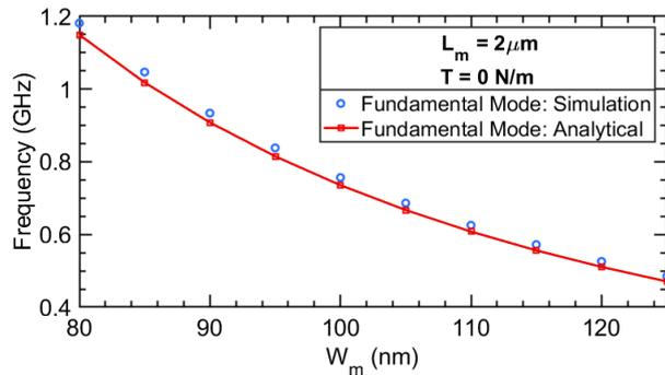
Fig. 3: Frequency vs  $W_m$  for a graphene membrane of  $L_m = 2\mu\text{m}$  under no tension. The analytical model (Eq.4) in red matches the FEM simulations in blue.
