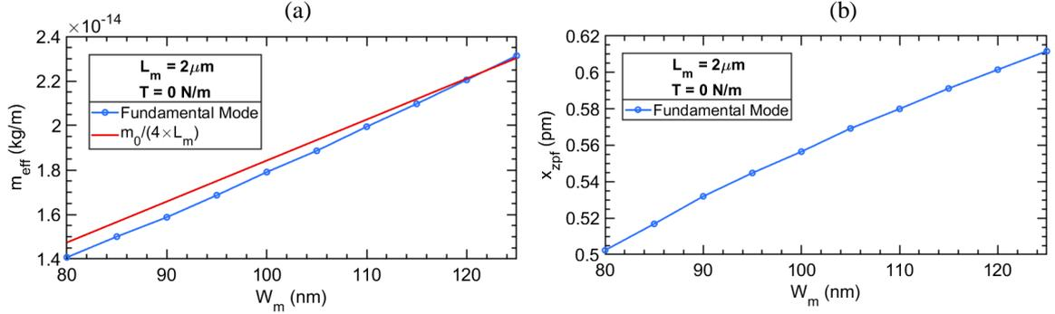
Fig. 4: (a)  $m_{eff}$  vs  $W_m$  for the first mode of the mechanical resonator. The red curve ( $\frac{m_0}{4 \times L_m}$ ) is the approximated effective mass of bridges. (b) Zero point motion amplitude as a function of  $W_m$ .
