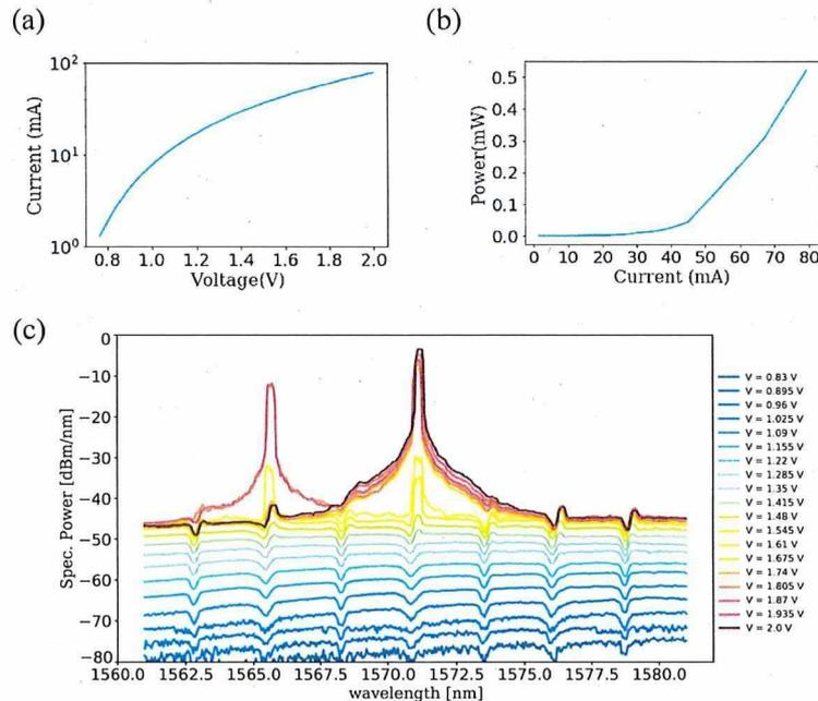
Fig. 2: (a) Current-voltage curve. For high bias voltages, a  $10\ \Omega$  series resistance is obtained. (b) waveguide-coupled optical power, showing a threshold current of 40 mA. (c) Optical spectrum for various amplifier bias voltages. The laser operates at 1571 nm, with a SMSR of 40dB
