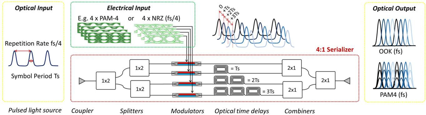
Fig. 1. Operation principle of an optical 4:1 serializer and modulator: For a target symbol rate  $R_s$ , a pulsed light source with a pulse width  $T_s$  (corresponding to the desired symbol rate) and a repetition rate at the quarter rate ( $R_s/4$ ) enters the optical chip. The light is divided equally over 4 branches where it is intensity modulated at  $fs/4$  and delayed over 0 to 3 symbol periods. After recombination, a waveform is achieved at the target  $R_s$  symbol rate.
