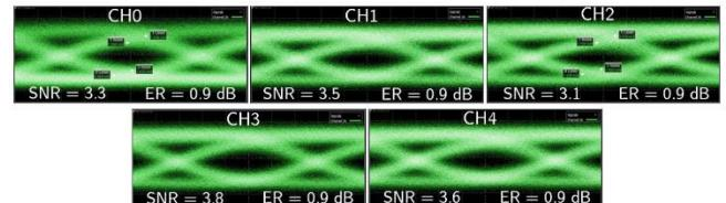
Fig. 5 Eye diagrams measured at 25 Gbit/s on the 5 channels of a WDM transmitter with  $W_{wg} = 600 \text{ nm}$  and  $L_{device} = 100 \mu m$  at 2.5 V<sub>pp</sub> and -1.2 V DC bias.
