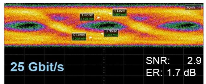
Fig. 2 Optical 2<sup>7</sup>-1 PRBS eye diagrams measured at 1560 nm, with a drive voltage of 2.5 V<sub>pp</sub> and a voltage bias of 2 V, at 25Gbit/s.
