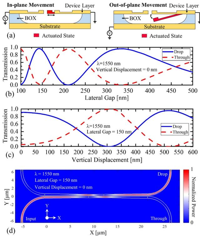
**Fig. 2.** (a) Possible actuation mechanisms for a suspended directional coupler. The simulated transmission in the drop and through ports of the coupler versus (b) the lateral air gap between the coupled waveguides and (c) the vertical displacement of one of the coupler’s arms at  $\lambda = 1550$  nm. (d) The electrical power profile in the coupler for a lateral gap of 150 nm and a vertical displacement of 0 nm at  $\lambda = 1550$  nm.
