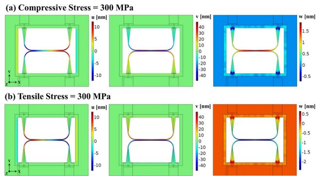
**Fig. 3.** Displacement field components for the suspended directional coupler under 300 MPa of (a) compressive stress and (b) tensile stress. The  $u$ ,  $v$ , and  $w$  correspond to the displacement field components in the X, Y, and Z directions, respectively.
