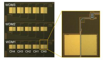
**Fig. 1.** Top-view microscope image showing the three WDM transmitters, each based on five graphene-Si EAMs and five second-order MRRs.
