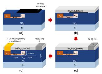
**Fig. 2.** Main steps of the process flow used to fabricate the graphene-Si EAMs: (a) graphene shaping, (b)  $Si(0.5 \text{ nm})/Al_2O_3$  (10 nm) deposition, (c) graphene contact, and (d) Si contact. The passivation layer on graphene helps in obtaining uniform and hysteresis-free performance. The Si waveguide is connected to a TE-mode fiber grating coupler.
