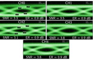
**Fig. 6.** Eye diagrams measured at 25 Gbit/s on WDM2 at  $2.5 \, V_{pp}$  and  $-1.2 \, V$  DC bias. The performance is uniform across the five channels. The dynamic extinction ratio is limited by the low modal overlap with graphene when using TE-polarized light.
