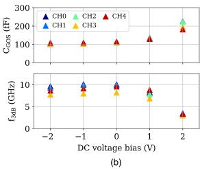
**Fig. 5.** (a) Electro-optical  $S_{21}$  (inset:  $S_{11}$ ) frequency response measured at 0 V DC bias on WDM2. The response is uniform across the five channels. (b) GOS capacitance and 3 dB bandwidth of WDM1 as a function of DC bias. The GOS capacitance increases at forward bias, causing a drop in 3 dB bandwidth. The ideal operating region is therefore at 0 V or low reverse bias.
