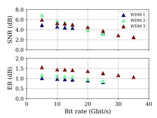
**Fig. 7.** SNR and dynamic ER as a function of bit rate. The SNR is higher than 3.0 up to 25 Gbit/s for all the WDM transmitters. The ER for WDM3 is higher than 1 dB up to 30 Gbit/s, due to the longer device length.
