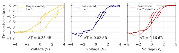
**Fig. 4.** Comparison of transmission curves, measured with a double-voltage sweep right after fabrication, between an unpassivated (yellow) and a passivated (blue) 25-μm-long graphene EAM. The unpassivated EAM shows hysteretic behavior, which is not present in the passivated EAM. The same measurement is repeated on the passivated EAM after two months (red), showing a small hysteresis that remains less pronounced compared to the unpassivated device.
