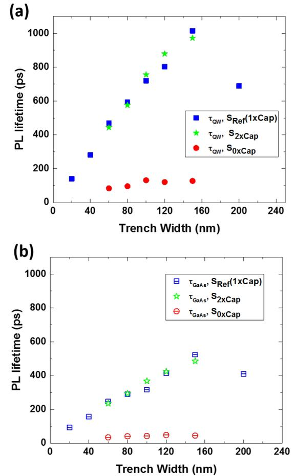
FIG. 5. Room-temperature PL lifetime from the reference sample ( $S_{ref}$ ) with 50 nm InGaP passivation layer, the sample without passivation layer  $S_{0 \times Cap}$  and the sample with 100 nm  $S_{2 \times Cap}$  passivation layer. a) Lifetime  $\tau_{QW}$  for QW PL emission and b)  $\tau_{GaAs}$  for GaAs.
