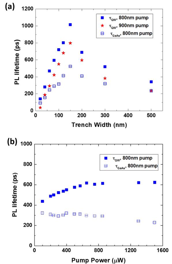
FIG. 4. a) PL lifetime versus trench width for the reference sample  $S_{Ref}$ , measured at room-temperature under 800 nm and 900 nm excitation wavelength respectively. The excitation power is 500  $\mu W$ . b) PL lifetime as a function of excitation power for a trench width of 80 nm.
