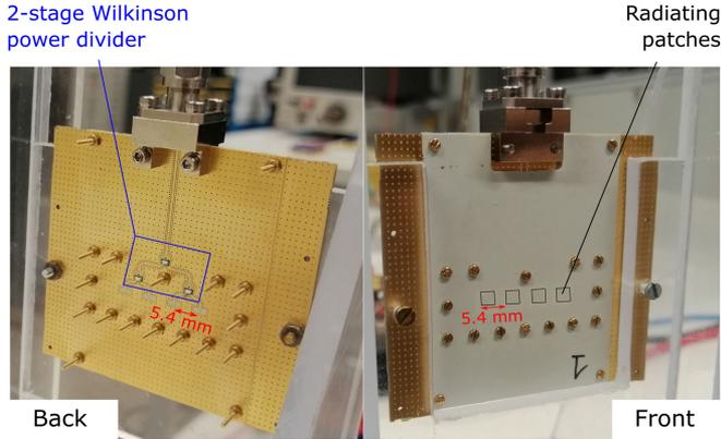
Fig. 6. Wilkinson-power-divider-fed 1×4 uniform linear antenna array covering the nr257/nr258 bands (24.25-29.5 GHz).
