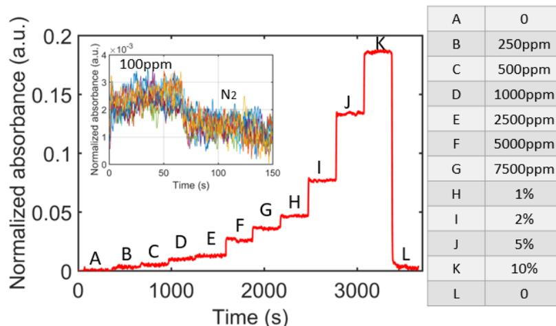
Figure 2: CO<sub>2</sub> sensing result, the concentrations from A to L are listed on the right, the inset shows the response to 100ppm CO<sub>2</sub>, with 10 identical measurements superimposed in one figure.
