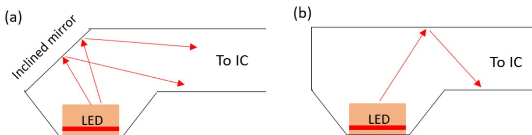
Figure 3: Coupling schemes from the LED die to the input waveguide, or from the output waveguide to the photodiode. The LED die has a dimension of  $L * W * H = 400 \mu\text{m} * 400 \mu\text{m} * 200 \mu\text{m}$ , and the absorption coefficient of the substrate is set to be  $20 \text{ cm}^{-1}$ , the photodiode used for simulation has the same dimensions as the LED.
