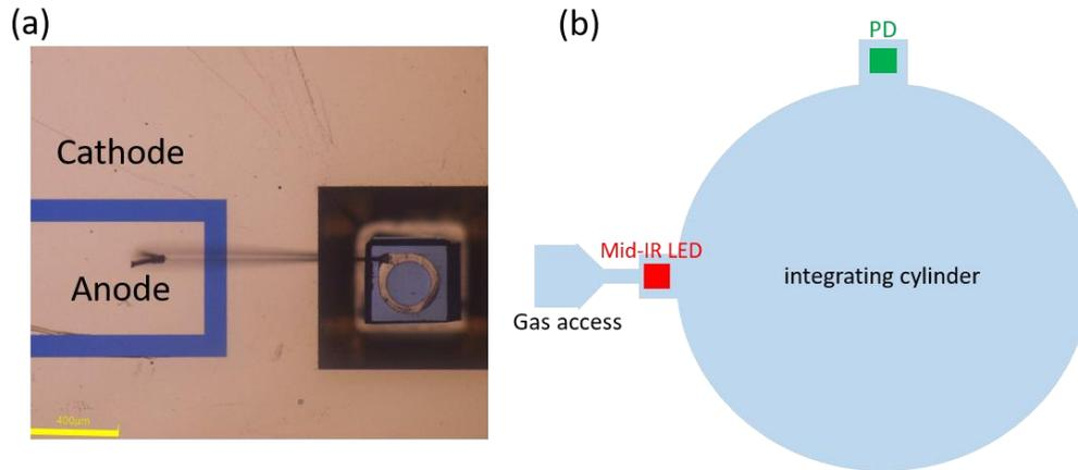
Figure 4: (a) Microscope image of the integrated LED on the top substrate, the LED die has a planar bottom contact and a ring top contact, the trench is 450 μm by 450 μm at the bottom, and the height of the trench is 250 μm, the thickness of the wire bond is 80 μm. (b) Proposed full sensor design, consisting of a Mid-IR LED, a photodiode, and an integrating cylinder.
