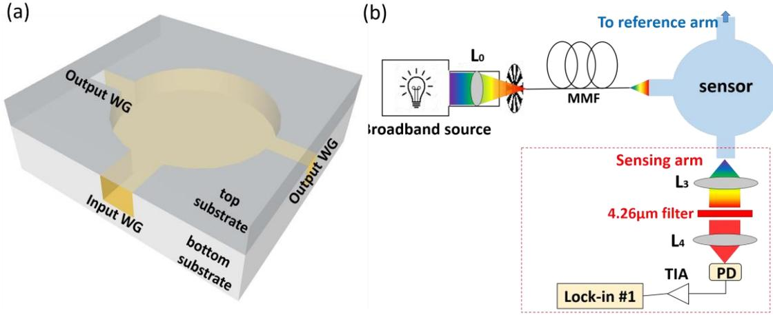
Figure 1: (a) 3D schematic of the integrating cylinder, the diameter and height of the cavity are 4mm and 300 $\mu$ m, respectively, the length and width of the access waveguides are 1mm and 200 $\mu$ m, respectively. (b) Experimental setup. L: lens MMF: multimode fiber, PD: photodiode, TIA: trans-impedance amplifier
