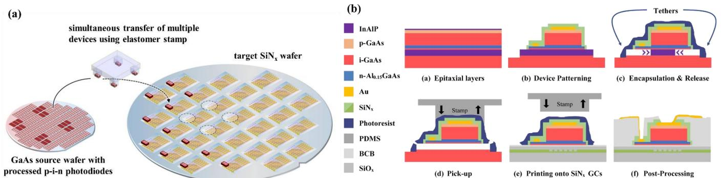
Fig. 1. Schematics of (a) micro-transfer printing on wafer-level scale and (b) the device fabrication and  $\mu\text{TP}$  process on a component level.
