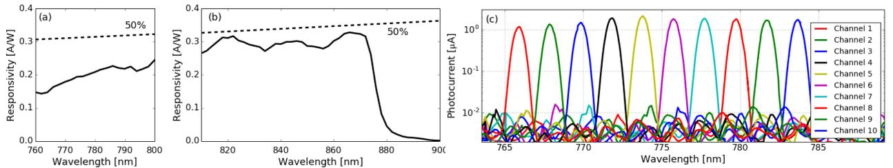
Fig. 3. The measured responsivity of the waveguide-coupled PD (a) from 760 nm to (b) 900 nm. (c) Shows the measured photocurrent of the AWG output PDs.
