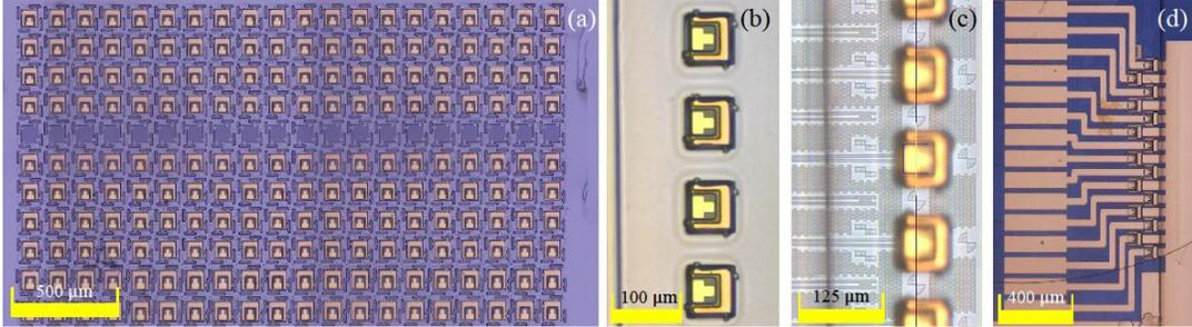
Fig. 2. Microscope images of (a) the source substrate with pre-processed PDs, (b) multi-PD pick-up on the PDMS stamp, (c) visual alignment and printing on top of the AWG channel output GCs and (d) the final interconnected system after post-processing (planarization, VIA access and metallization).
