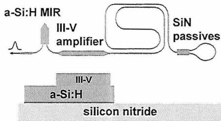
Schematic of the envisioned anti-colliding mode-locked laser
