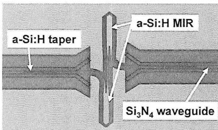
Fabry-Pérot interferometer using two MIRs as cavity mirrors.
