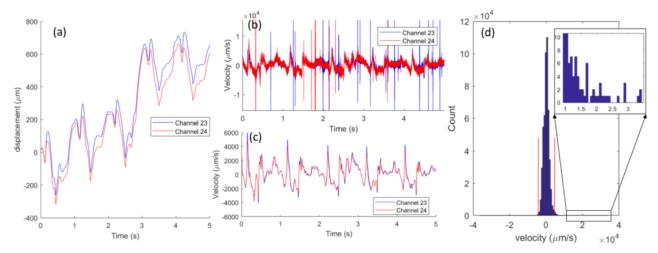
Figure 3. (a) Measured displacement signal of carotid pulses with help of RR patches at two adjacent locations with a spacing of 5 mm. (b) The velocity values of the pulses (without filter). (c) The velocity values of the pulses (with a 30 Hz lowpass filter). (d) Histogram of unfiltered velocity values.
