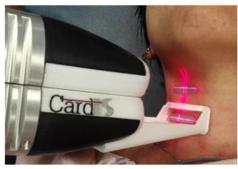
Figure 1. (a) The CARDIS handheld LDV sensor with 2 x 6 beams at 1550 nm. The LDV sensor is developed in CARDIS project. (b) The measurement position of the LDV sensor for local-carotid PWV measurement. Reproduced from [3]
