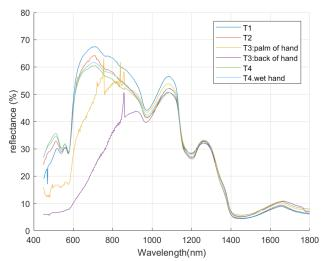
Figure 7. The reflectance of light from hand skins of four different candidates with different skin colors.
