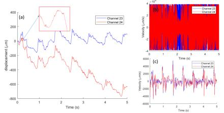
Figure 5. (a) Measured displacement signal of the carotid pulse at two adjacent locations with a spacing of 5 mm, without RR patches. (b) The velocity values of the pulses (without filter). (c) The velocity values of the pulses (with 30 Hz lowpass filter)
