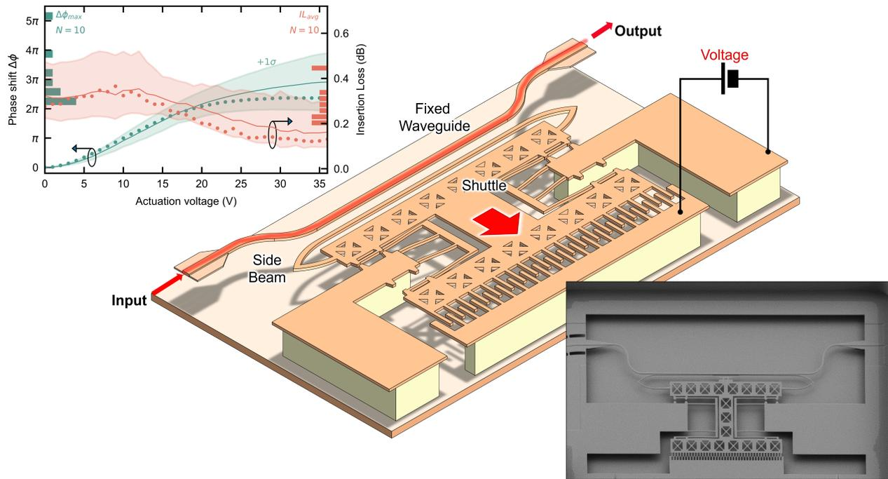
Figure 3.<sup>14</sup> The phase shift is induced by a narrow beam of silicon positioned parallel to the waveguide, where the distance between the beam and the waveguide can be adjusted using an electrostatic comb drive. The 50  $\mu\text{m}$  long device achieves a  $2\pi$  phase shift for an actuation of 20 V.
