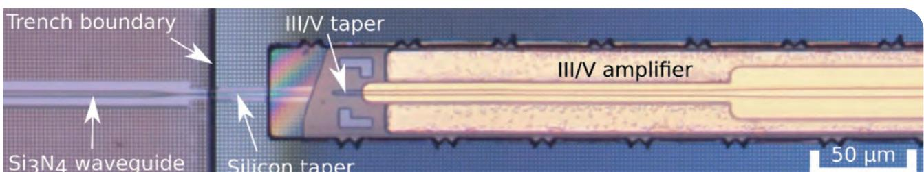
► Figure 2. Microscope image of the micro-transfer printed coupon on top of the two-stage taper coupling structure.
