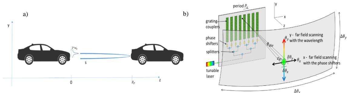
Figure 1a) LiDAR in forward looking automotive b) Beam steering with a 1-dimensional optical phased array (from [1])
