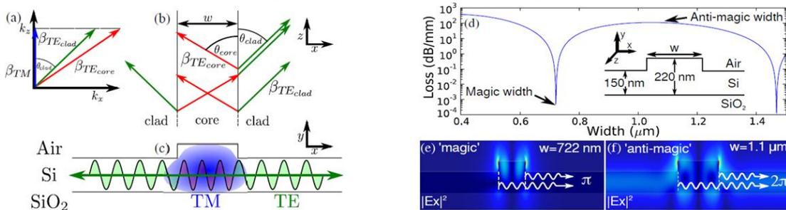
Figure 2 Lateral leakage in rib waveguides (taken from [2])
