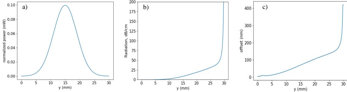
Figure 5 a) desired output profile b) corresponding radiation strength required c) antenna design, offset value at each position  $y$
