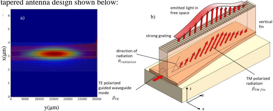
Figure 6 a) simulation of antenna design b) conceptual 3D drawing of antenna design concept
