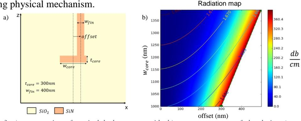
Figure 3 a) cross-section of vertical leakage waveguide b) parameter sweep of the device,  $t_{core} = 300\text{nm}$ ,  $w_{fin} = 400\text{nm}$
