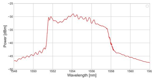
(e) Optical spectrum of the mode-locked laser.
