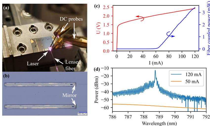
Fig. 2. (a) Measurement setup showing light emission at a driving current of 70 mA, visible by naked eye as red light. (b) Two printed lasers on Si before post-printing-processing. (c) Fiber-coupled power and bias voltage as a function of driving current. (d) Spectrum at 120 mA driving current (blue line) measured with 33 pm resolution compared to the ASE spectrum at 50 mA (orange line).
