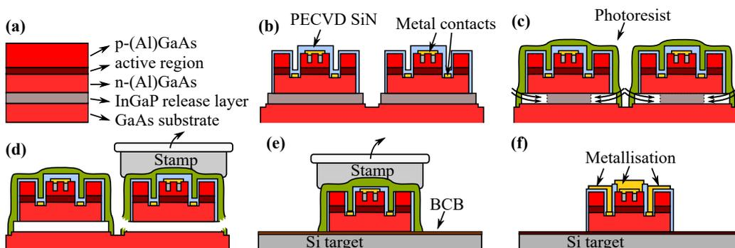
Fig. 1. Fabrication of transfer printed lasers: (a) Epitaxial layer stack. (b) Coupon fabrication, including metal contacts. (c) Encapsulation of laser coupons in photoresist and selective under-etch of InGaP release layer through holes in the photoresist. (d) Pick-up of laser coupon using a polymer stamp. (e) Printing of laser coupon on Si target substrate with a thin BCB adhesion layer. (f) Subsequent encapsulation removal and metallisation of contact pads.
