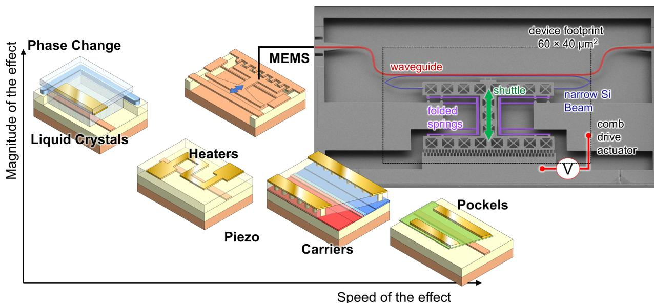
Figure 4. Electro-optic actuation mechanisms, classified by the speed of the effect and the magnitude. The stronger the effect, the shorter and more compact the phase shifter can be implemented. Inset: A MEMS Phase shifter developed in the MORPHIC project.<sup>23</sup>
