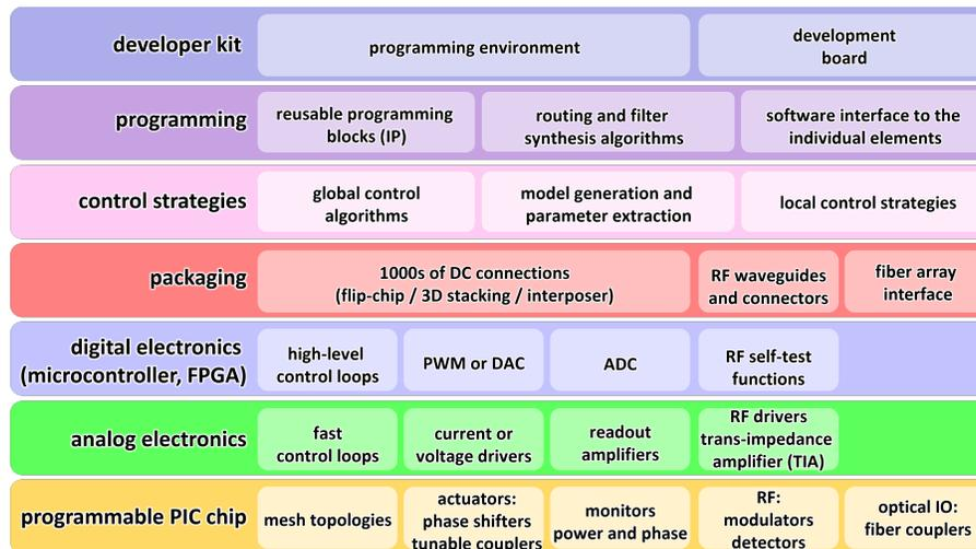
Figure 3. Technology stack for programmable photonics.<sup>4,6</sup> To realize a programmable photonics system, one needs to combine the photonic chip with analog and digital driver electronics and software layers.
