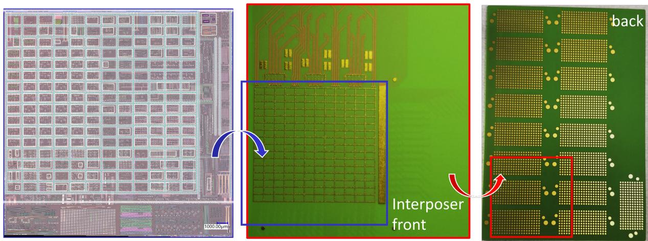
Figure 5. Interposer technology developed in the MORPHIC project.<sup>46</sup> The silicon photonics chip can have up to 3305 electrical connections on a fixed grid. A ceramic interposer breaks out these bond pads to a much wider pitch compatible with standard printed circuit board technology. The interposer also supports up to 24 high-speed connections for modulators and photodetectors.
