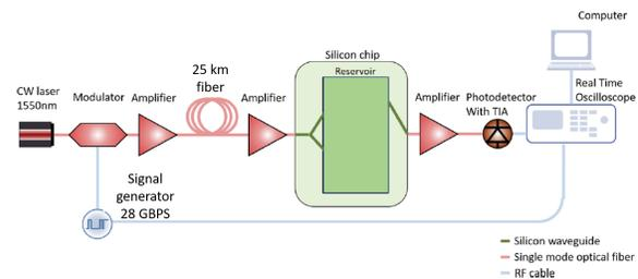
Fig. 1. Schematic illustration of the setup used in the experiment.
