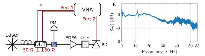
**FIG. 4**. (a) Schematic overview of the measurement setup used to perform the frequency domain measurements. (PM = Power Meter, EDFA = Erbium Doped Fiber Amplifier, OTF = Optical Tunable Filter, PD = Photodiode, VNA = Vector Network Analyzer, DUT = Device Under Test) (b) Measured  $|S_{21}|$  as a function of the modulation frequency, obtained by using the setup in (a). The measurement hits the noise floor around 55 GHz.
