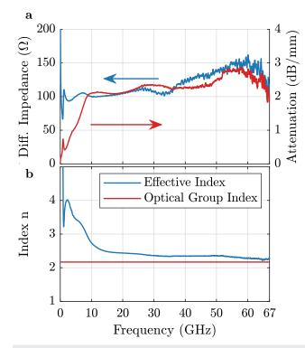
**FIG. 3.** High speed electrical characteristics. [(a) left] The characteristic impedance of the differential transmission line as a function of the modulation frequency. [(a) right] Electrical attenuation as a function of the modulation frequency. (b) Effective electrical index as a function of the modulation frequency; the red line is the target optical group index.
