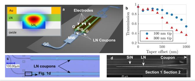
FIG. 1. (a) Schematic image of the complete device. (inset) Overview of the hybrid LN-on-SiN mode profile. Both the SiN and the LN layers are 300 nm thick. The SiN waveguide is 1  $\mu$ m wide. (b) Simulation results of the 45  $\mu$ m long bilinear taper as a function of the taper tip width and alignment offset. (c) Microscope image of the printed LN coupons on SiN waveguides. (d) SEM image of the LN taper.
