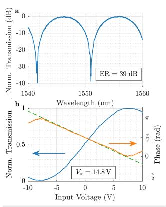
**FIG. 2.** Low frequency measurement results. (a) Normalized wavelength sweep of the MZI structure, the free spectral range is 9.5 nm and the extinction ratio is 39 dB. (b) Output power as a function of the applied voltage (blue line). Extracted phase change depending on the applied voltage (orange line), fitted linear phase change resulting in a  $V_{\pi}$  of 14.8 V (green striped line).
