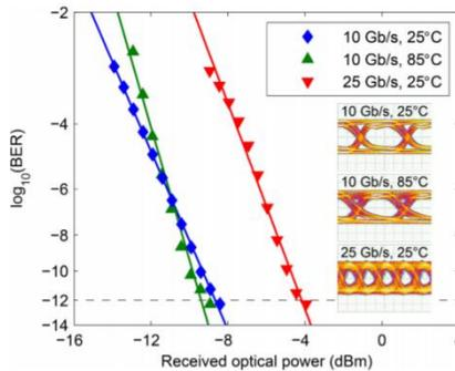
**Fig. 6.11.** Measured BER versus received optical power for a 5- $\mu\text{m}$  oxide aperture diameter HC-VCSEL with similar resonance wavelength as HC-VCSEL C at data rates up to 25 Gbit/s at 25  $^{\circ}\text{C}$  and 10 Gbit/s at 85  $^{\circ}\text{C}$ . Insets: Corresponding optical eye diagrams (scales: 100 mV/div and 20 ps/div). Reproduced from [4].
