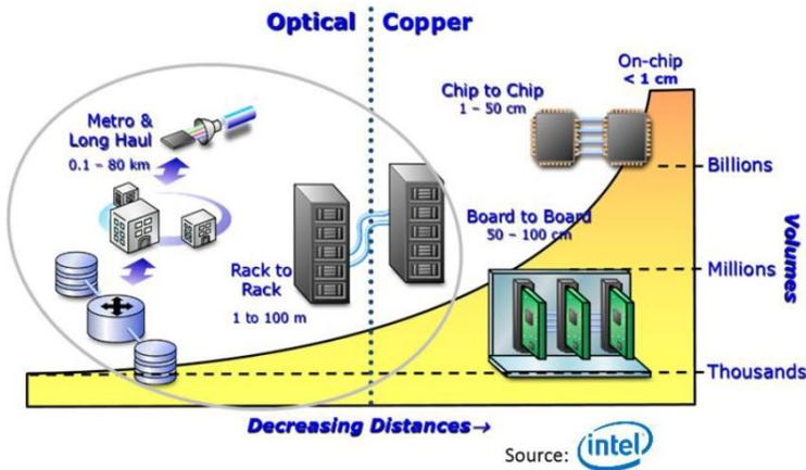
Fig. 1.2 Optical interconnects roadmap in data communication networks.
