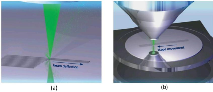
**Fig. 4.3** (a) Illustration of conventional e-beam writing mode. The beam is deflected while the stage is stationary, resulting in a stitching error of several nm. (b) FBMS mode. The beam is fixed while the stage is moving. Reproduced from [7]
