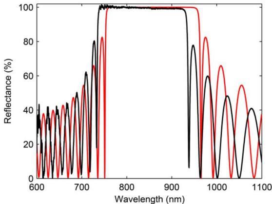
**Fig. 3.2** Simulated (red) and measured (black) spectral reflectance for the 20-pair SiO<sub>2</sub>/Ta<sub>2</sub>O<sub>5</sub> dielectric DBR on Si substrate, reproduced from [1].
