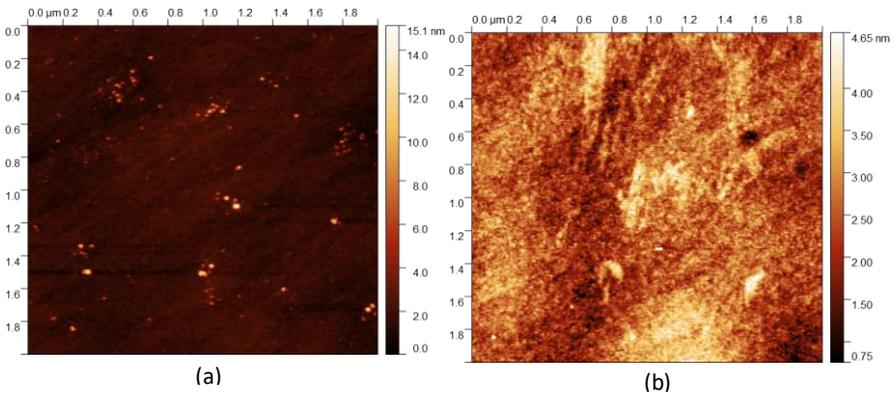
**Fig 5.5** AFM image of the final GaAs surface after etching of GaAs in citric acid for 20 sec and AlAs in HCl:H<sub>2</sub>O (1:1) for 1 min (a) before treatment with the digital wet etch and (b) after treatment with the digital wet etch.
