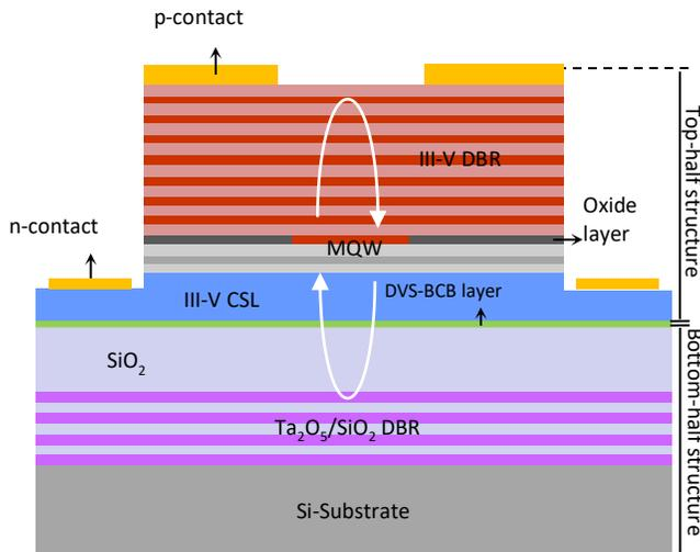
**Fig. 3.1** Schematic cross section of the  $845\text{-nm}$ -wavelength Gen1 HC VCSEL.
