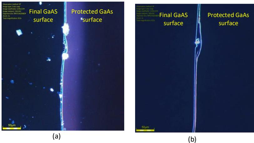
**Fig. 5.4** Dark field microscope image of the final GaAs surface after etching of GaAs in citric acid for 20 sec and AIAs in HCl:H<sub>2</sub>O (1:1) for 1 min (a) before treatment with the digital wet etch and (b) after treatment with the digital wet etch
