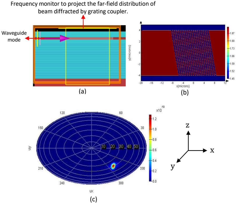
**Fig. 3.14** (a) Cross-section view ( $xz$ -plane) of simulation setup (b) Index profile of SiN grating with waveguide ( $xy$ -plane) (grating teeth are tilted at an angle of 20 degree) (c) Far field projection of the beam diffracted by the grating coupler
