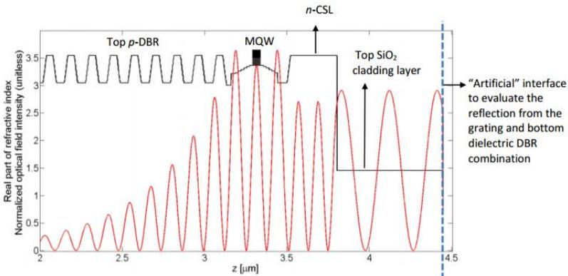
**Fig. 3.12** Refractive index distribution (black line) and simulated resonant optical field intensity (red line) along the  $z$ -axis of a 855-nm-wavelength VCSIL.
