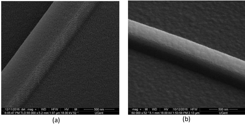
**Fig. 4.9** Sidewall roughness of the waveguide after dry etching and removal of the e-beam resist at (a) a reflow temperature of 143°C for 2 min and (b) a reflow temperature of 150°C for 2 min (A thin gold layer is deposited on the top surface to reduce the charging during SEM imaging).
