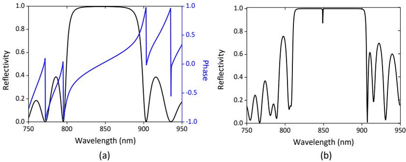
**Fig. 2.3** (a) Reflectivity and phase as a function of the wavelength for 24 pairs of an  $\text{Al}_{0.12}\text{Ga}_{0.88}\text{As}/\text{Al}_{0.90}\text{Ga}_{0.10}\text{As}$  DBR with air interface, (b) full VCSEL cavity dip position at 845 nm. The single narrow longitudinal resonance is seen at 845 nm.
