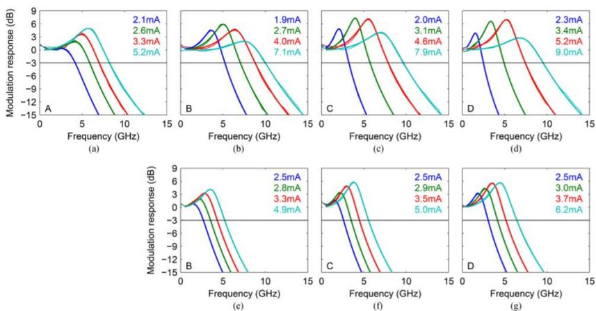
**Fig. 6.8.** Small-signal modulation response at 25 °C (a)-(d) and 85 °C (e)-(g) for HC-VCSELs A-D at indicated bias currents. The maximum 3 dB modulation bandwidth is reached at the highest bias currents indicated. Reproduced from [4].
