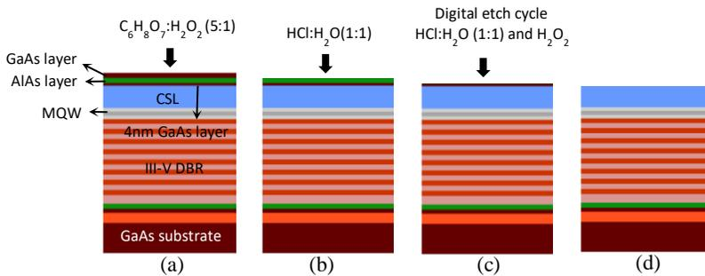
**Fig. 5.7** Sacrificial layer etching prior to bonding: (a) 30 sec dip in HCl:H<sub>2</sub>O (1:1) to remove the native oxide, (b) etching of the GaAs layer in C<sub>6</sub>H<sub>8</sub>O<sub>7</sub>:H<sub>2</sub>O<sub>2</sub> (5:1) solution for 20 sec, (c) etching of the AlAs layer in HCl:H<sub>2</sub>O (5:1) solution for 1 min, (d) 3 cycles of digital etching in HCl:H<sub>2</sub>O (1:1) and H<sub>2</sub>O<sub>2</sub> solution.
