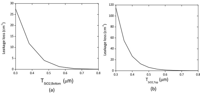
**Fig. 3.6** Oxide cladded  $5.5 \mu\text{m} \times 300 \text{ nm}$  SiN waveguide leakage loss as a function of (a) bottom oxide cladding layer thickness (855 nm wavelength, TE polarization), and (b) top oxide cladding layer thickness (855 nm wavelength, TE polarization).
