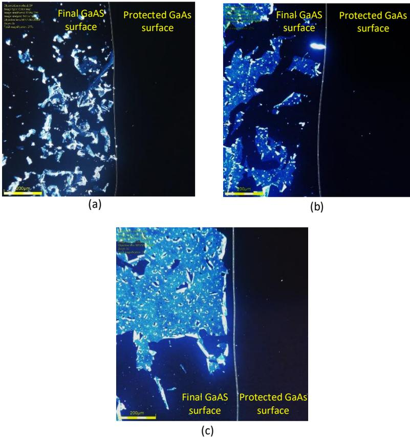
**Fig. 5.3** Dark field microscopic image of the final GaAs surface after etching of GaAs in citric acid for (a) 20 sec (b) 40 sec and (c) 60 sec . The AlAs layer is etched in HCl:H<sub>2</sub>O (1:1) for 1 min.
