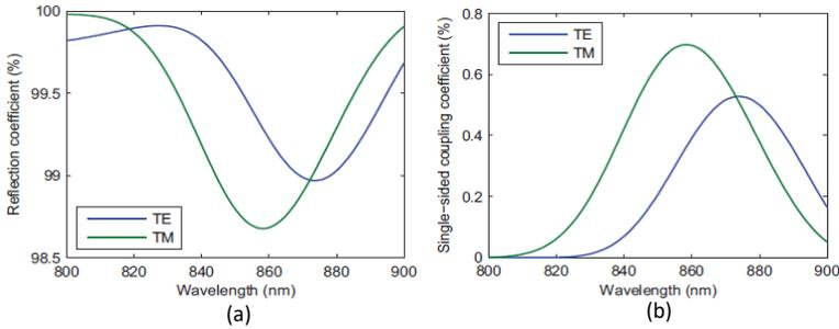
**Fig. 5** (a) Simulated reflection coefficient and (b) single-sided coupling coefficient of the intra-cavity grating/dielectric DBR combination as a function of wavelength for TE and TM polarizations. (grating period = 530 nm, DC = 50%)
