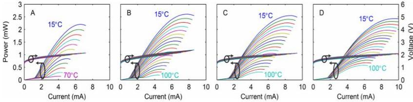
**Fig. 6.3** Output power and voltage versus current for HC-VCSELs A–D measured at ambient temperatures ranging from 15 to 100  $^{\circ}\text{C}$  in steps of 5  $^{\circ}\text{C}$ , reproduced from [4].
