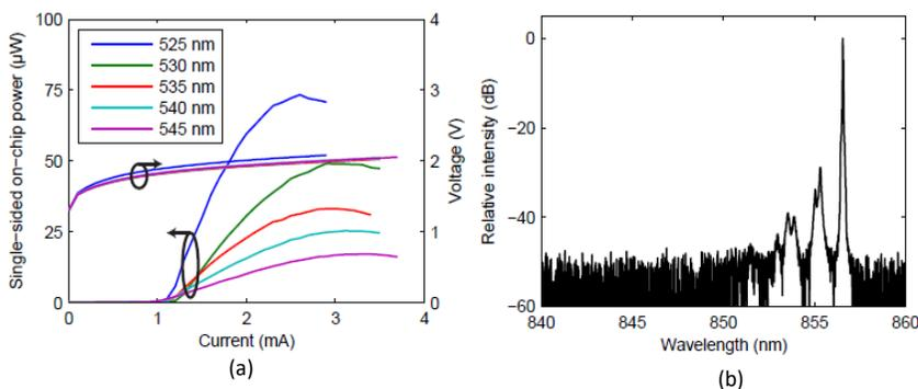
**Fig. 6.13** (a) Waveguide-coupled light-current-voltage characteristics for 5 μm oxide-aperture diameter VCSILs with intra-cavity grating periods ranging from 525 - 545 nm (after gold deposition on the surface). (b) Spectrum for the 525 nm device operated at 2.5 mA.
