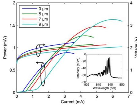
**Fig. 6.2** Measured light-current-voltage characteristics for hybrid-cavity VCSELs with oxide aperture diameters of 3–9  $\mu\text{m}$ . Inset: spectrum for a 7  $\mu\text{m}$  aperture VCSEL operated at 3.0 mA. Reproduced from [1]
