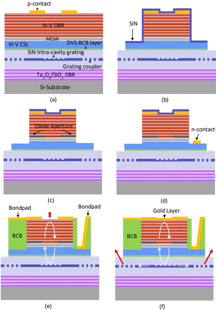
**Fig. 5.16** The process steps for hybrid-cavity Gen2 VCSIL fabrication include: (a) p-contact deposition, (b) mesa etching followed by deposition of SiN, (c) oxide aperture formation after opening of SiN on the mesa sidewalls, (d) n-contact deposition, (e) planarization with DVS-BCB, and deposition of bondpads and (f) deposition of a gold reflector
