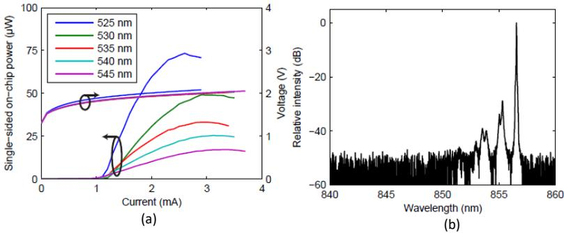
**Fig. 7** (a) Waveguide-coupled light-current-voltage characteristics for  $5 \mu\text{m}$  oxide-aperture diameter VCSILs with intra-cavity grating periods ranging from  $525 - 545$  nm (after gold deposition on surface). (b) Spectrum for the  $525$  nm device operated at  $2.5$  mA.
