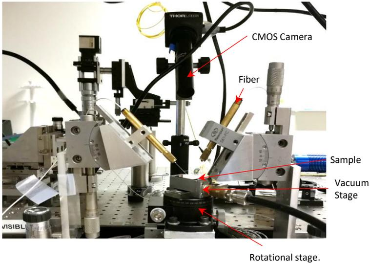
**Fig. 4.12** Vertical setup to measure waveguide losses.
