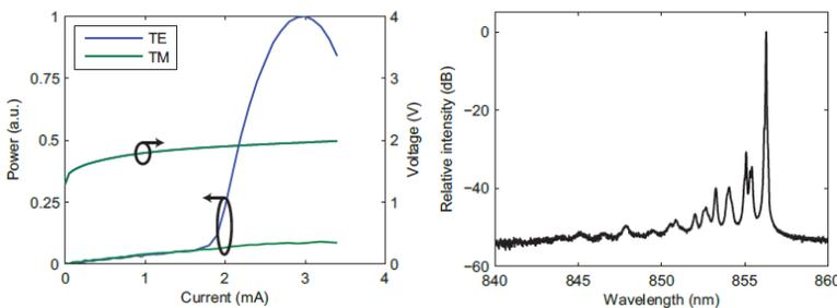
**Fig. 6.12.** (a) Polarization-resolved surface-emitted light-current-voltage characteristics for a 5  $\mu\text{m}$  oxide-aperture diameter VCSIL with 545 nm intra-cavity grating period and 50% DC (prior to gold deposition on the surface). (b) Surface emission spectrum for the same device operated at 2.5 mA.
