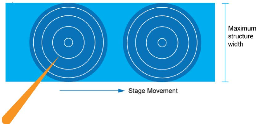
**Fig. 4.5** Circle generator pattern for FBMS area.
