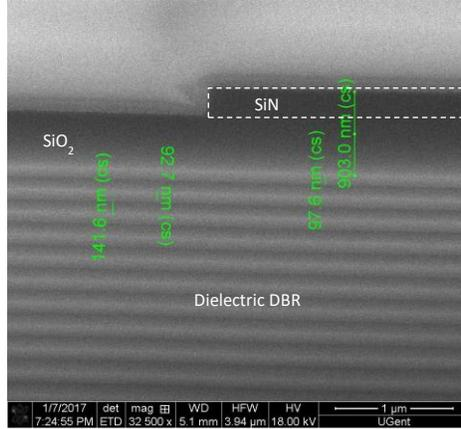
**Fig. 4.10** FIB CS image of the waveguide after reflow at 143°C for 2 min.
