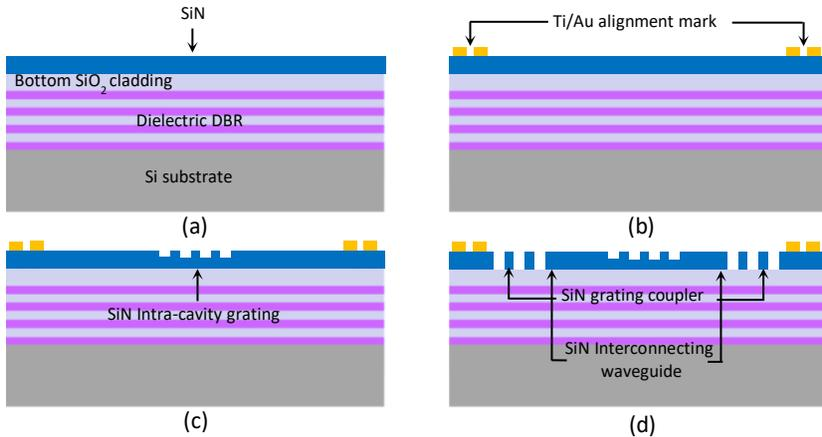
**Fig. 4.6** Schematic for ebeam writing of SiN PIC: (a) SiN and SiO<sub>2</sub> cladding layer on dielectric DBR (b) Ti/Au alignment marks (c) SiN intra-cavity grating and (d) SiN grating coupler and interconnecting waveguides.
