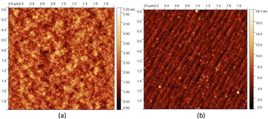
**Fig 5.6** AFM image of (a) Ta<sub>2</sub>O<sub>5</sub>/SiO<sub>2</sub> DBR surface and (b) GaAs surface without any etch.
