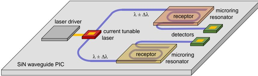
**Fig. 1.1** Multi-DoF (degree of freedom) sensor on chip, reproduced from [8].
