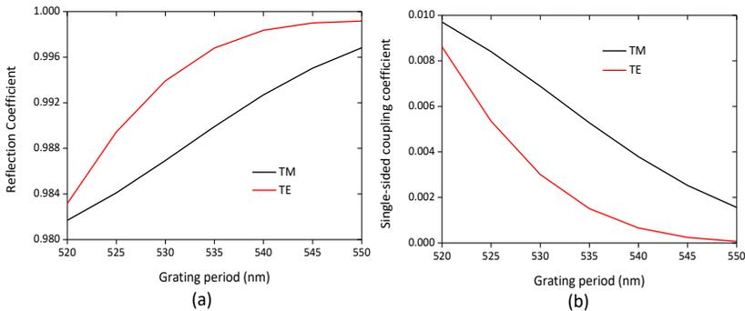
**Fig. 3.9** (a) Reflection and (b) single-sided coupling coefficient as a function of intra-cavity grating period for TE and TM polarizations at a resonance wavelength of 855 nm. Parameters of the simulations are  $2w = 4.7 \mu\text{m}$ , SiN waveguide core thickness = 300 nm,  $T_{\text{SiO}_2, \text{Bottom}}$  thickness = 610 nm, grating groove depth = 30 nm, and grating duty cycle = 50%.
