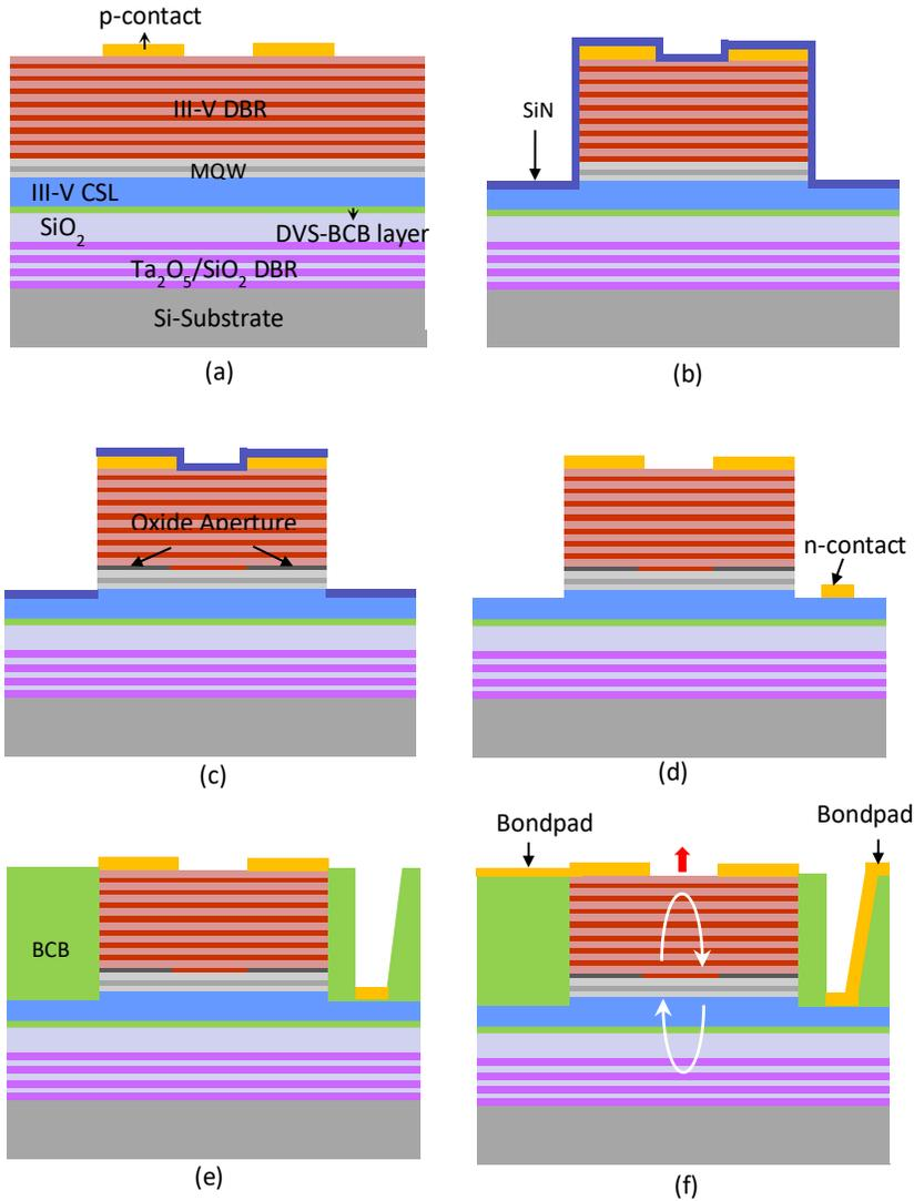
**Fig. 5.14** The process steps for hybrid-cavity GEN1 VCSEL fabrication includes: (a) p-contact deposition, (b) mesa etching followed by deposition of SiN, (c) oxide aperture formation after opening of SiN on mesa side walls, (d) n-contact deposition, (e) planarization with DVS-BCB, and (f) deposition of bondpads.
