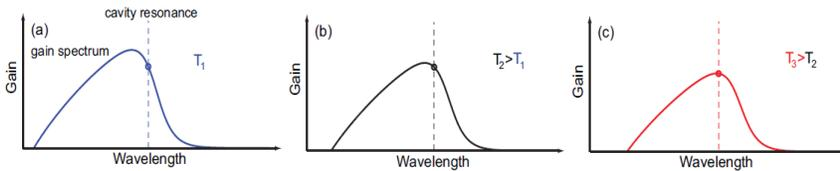
**Fig. 2.5:** Resonance/gain peak detuning with increasing temperature.
