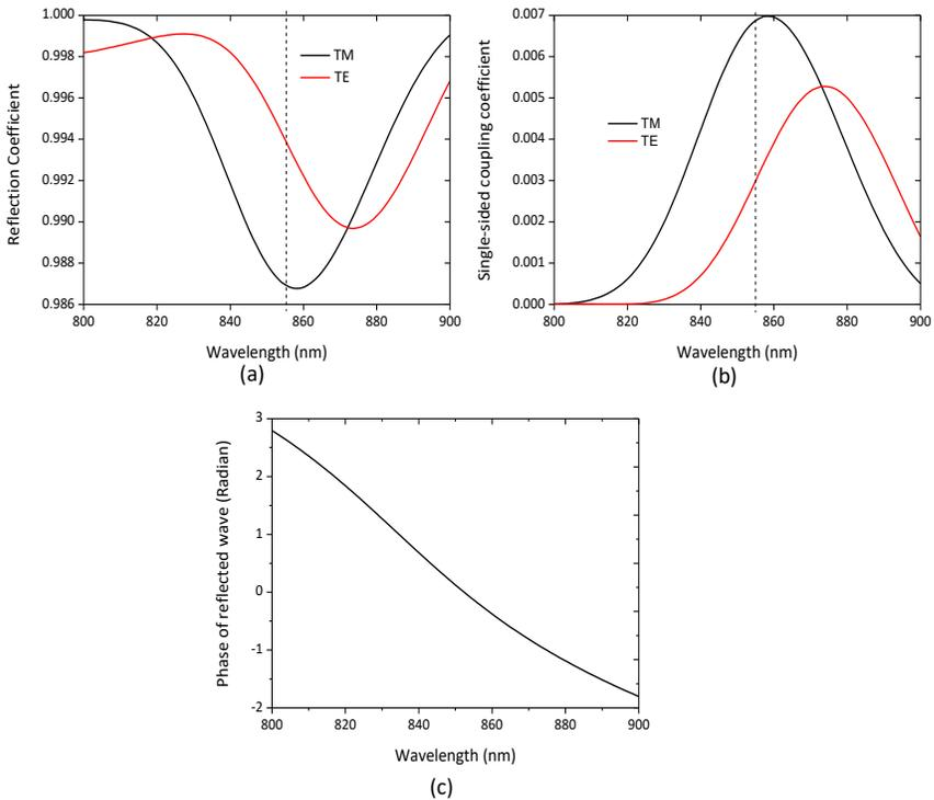
**Fig. 3.8** (a) Reflection coefficient as a function of wavelength for TE and TM polarization. (b) Single-sided coupling coefficient as a function of wavelength for TE and TM polarization. (c) Phase of the reflected wave for TE polarization. Parameters of the simulations are  $2w = 4.7 \mu\text{m}$ , grating period = 530 nm, SiN waveguide core thickness = 300 nm,  $T_{\text{SiO}_2, \text{Bottom}}$  thickness = 610 nm, grating groove depth = 30 nm, and grating duty cycle = 50%.
