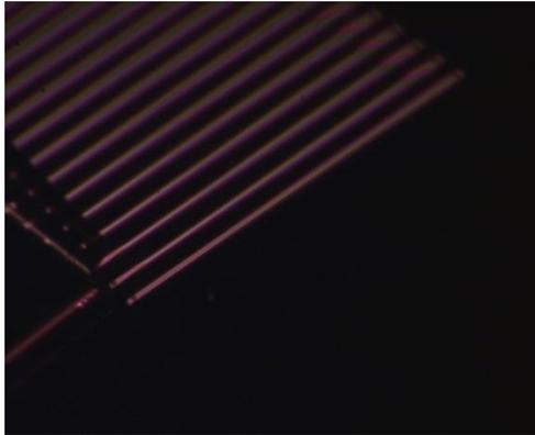
**Fig. 4.13** Sample rotated at 305 degree and an optical fiber rotated at 36 degree to couple the light into the SiN waveguide.
