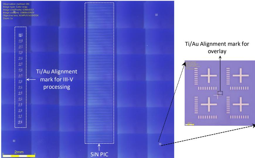
**Fig. 4.11** Microscope image of a SiN PIC.
