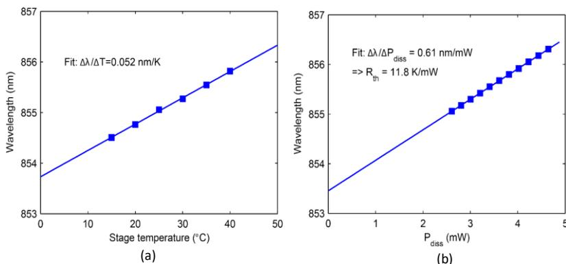
**Fig. 6.14** (a) Wavelength of the fundamental mode versus stage temperature at 25 °C for HC-VCSILs with oxide aperture of 5 μm with fits to extract the thermal impedance. (b) Wavelength of the fundamental mode versus dissipated power at 25 °C for HC-VCSILs with oxide aperture of 5 μm with fits to extract the thermal impedance.
