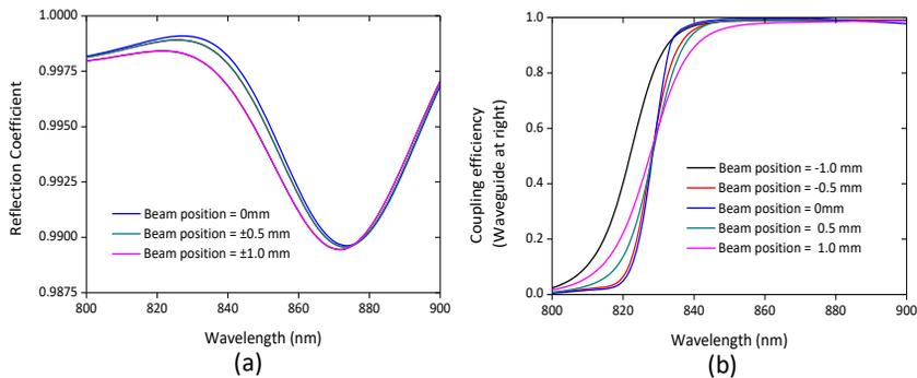
**Fig. 3.11** (a) Reflection coefficient and (b) right-hand-side waveguide coupling efficiency, as a function of alignment between the Gaussian beam center relative to the grating region center, in the direction perpendicular to the grating lines. The grating region center is considered as the beam position = 0. Parameters of the simulations are  $2w = 4.7 \mu\text{m}$ , grating period = 530 nm, SiN waveguide core thickness = 300 nm, grating groove depth = 30 nm, and grating duty cycle = 50%.
