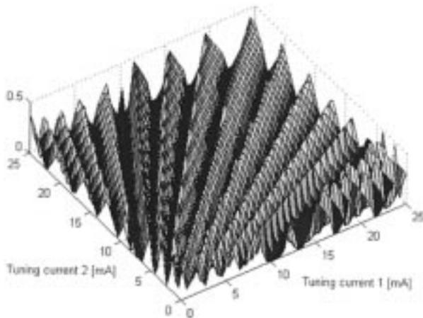
Fig. 3. Normalized threshold gain difference ( $\Delta(\Gamma g_{\text{th}}L)$ ) between main and sidemode as a function of the two tuning currents.
