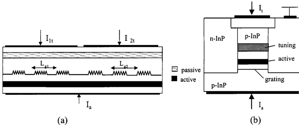
Fig. 1. Schematic structure of a  $\lambda/4$ -shifted (S)SG TTG laser. (a) Longitudinal/transverse cross section. (b) Lateral/transverse cross section.
