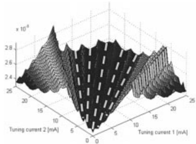
Fig. 4. Threshold gain (in  $\mu\text{m}^{-1}$ ) as a function of the two tuning currents. The dashed lines indicate lines along which a minimum gradient in threshold gain is obtained.
