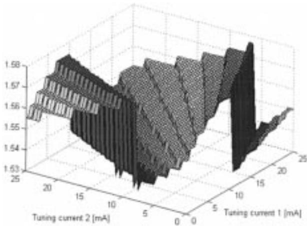
Fig. 2. Three-dimensional view of the wavelength (in  $\mu\text{m}$ ) as a function of the two tuning currents.
