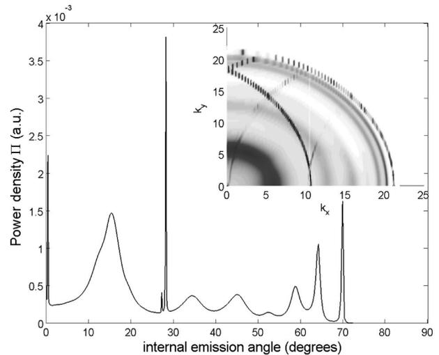
Fig. 8. Simulated power per unit solid angle along the  $x$  axis as a function of the angle in the highest-index medium. Inset: contour plot of the simulated power per unit solid angle in  $\mathbf{k}_\parallel$  space.
