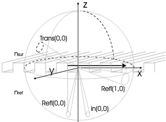
Fig. 5. Solid-angle transformation due to refraction and diffraction.
