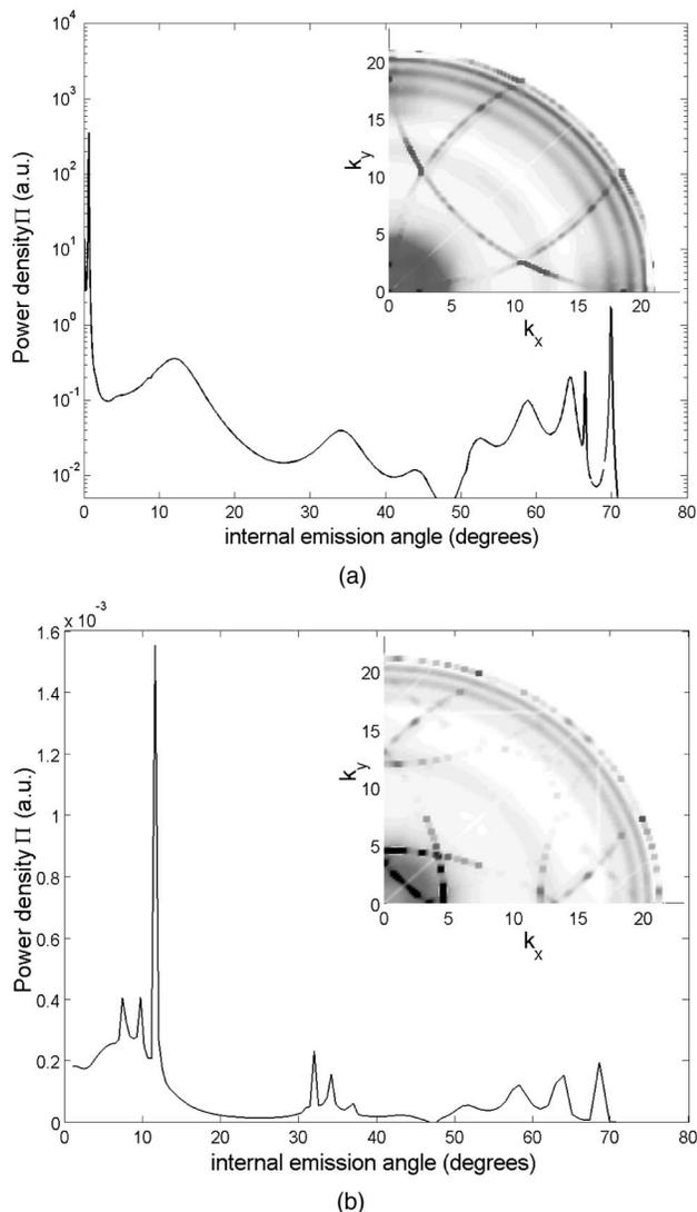
Fig. 10. Simulated power per unit solid angle along the  $x$  axis as a function of the angle in the highest-index medium. Inset: contour plot of the simulated power per unit solid angle in  $\mathbf{k}_{\parallel}$  space. (a) 2D partially metallized air-semiconductor square lattice grating of depth 90 nm, fill factor 0.5, and period 300 nm; (b) 2D partially metallized air-semiconductor square lattice grating of depth 90 nm, fill factor 0.5, and period 390 nm.
