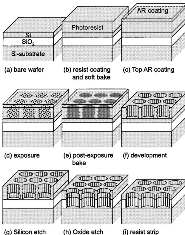
Fig. 3. Fabrication process with deep UV lithography in SOI.
