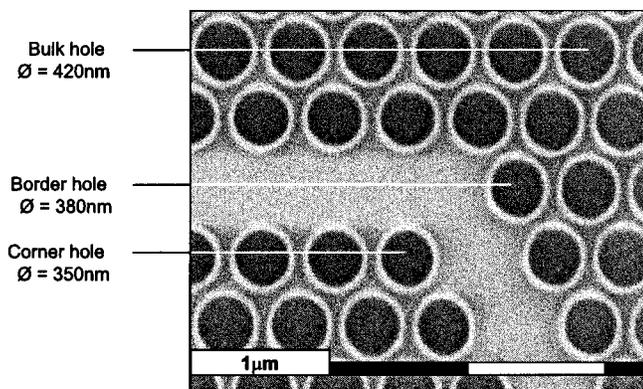
Fig. 7. Measurement of OPEs: 530 nm pitch. Although not noticeable on first sight, the holes in the corners are 70 nm smaller than the holes in the bulk of the lattice.
