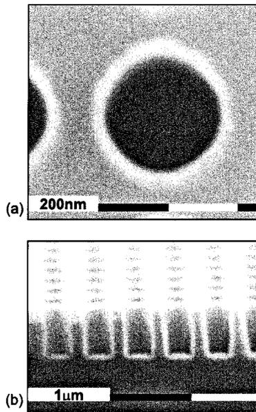
Fig. 4. Top-down view and cross section of etched holes in SOI. Pitch is 500 nm, hole size is 350 nm.
