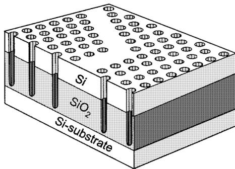
Fig. 1. Schematic drawing of a photonic crystal slab waveguide in silicon-on-insulator. The light is confined in the top silicon layer by total internal reflection, while horizontally it is confined by the photonic crystal holes.
