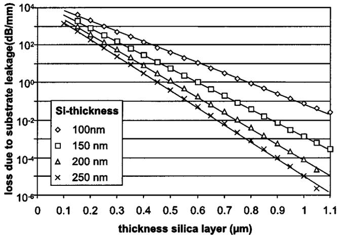
Fig. 2. Semi-log graph of the substrate loss in dB/mm as a function of silica layer thickness for four different values of silicon layer thickness.
