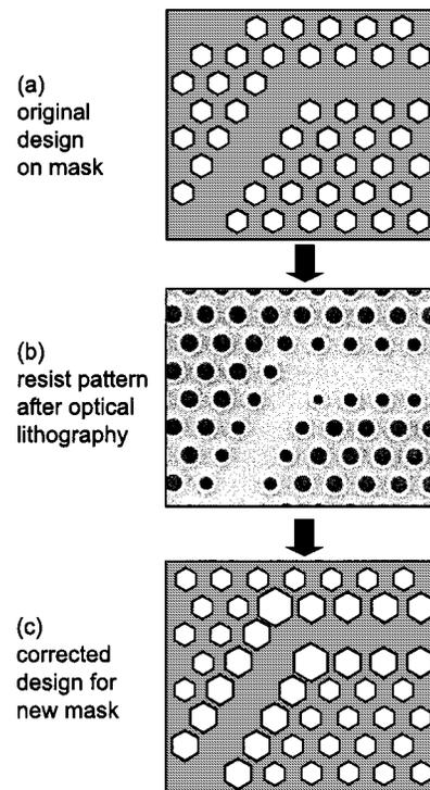
Fig. 6. Exaggerated illustration of OPEs. Although the holes on the reticle are all of the same size (a), the holes in the bulk of the lattice print different than the holes near the waveguide (b), so to correct for this OPC should be added to the mask (c).
