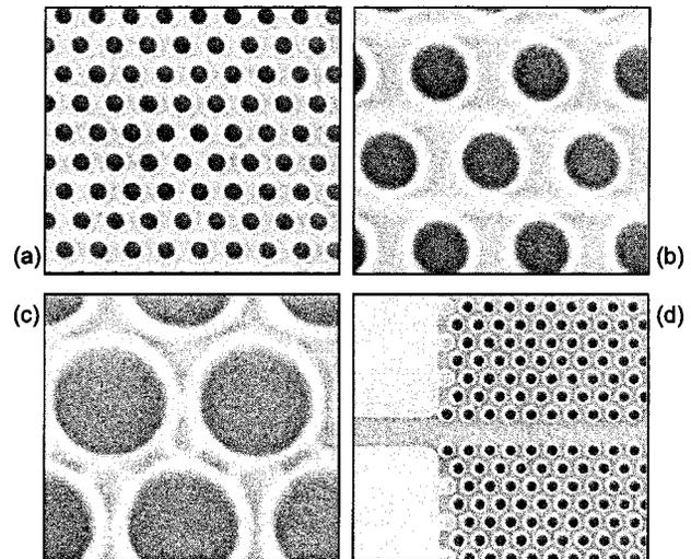
Fig. 5. Resist patterns of superdense holes in a triangular lattice. (a), (b) Pitch = 500 nm, hole diameter = 300 nm. (c) Pitch = 500 nm, Hole Diameter = 430 nm, resist channeling between holes. (d) Photonic crystal waveguide, Pitch = 460 nm, Hole diameter = 280 nm.
