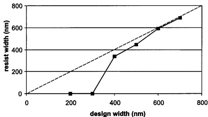
Fig. 8. Measurements of line-hole bias. Resist line width as a function of design line width of a narrow line when printed at the dose-to-target of a superdense triangular lattice (500-nm pitch, 300-nm hole size). The dashed line indicates features printed on target.
