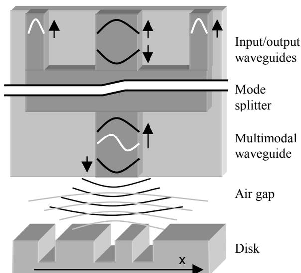
**Figure 1: Schematic view of the PIC, waveguide and disk.**
