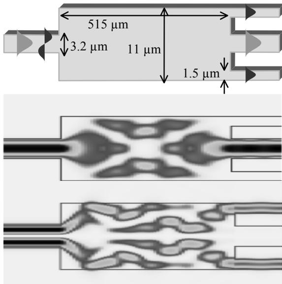
**Figure 3a: Mode splitter dimensions**
