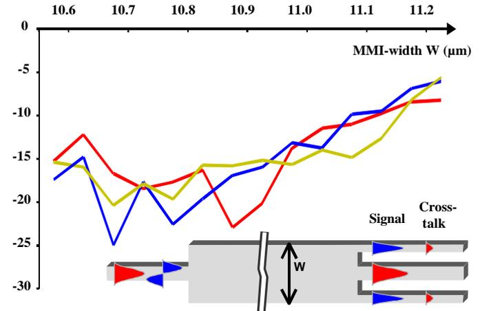
Figure 7: Measured crosstalk from the zeroth order mode to the output of the first mode, for a range of components with varying MMI width
