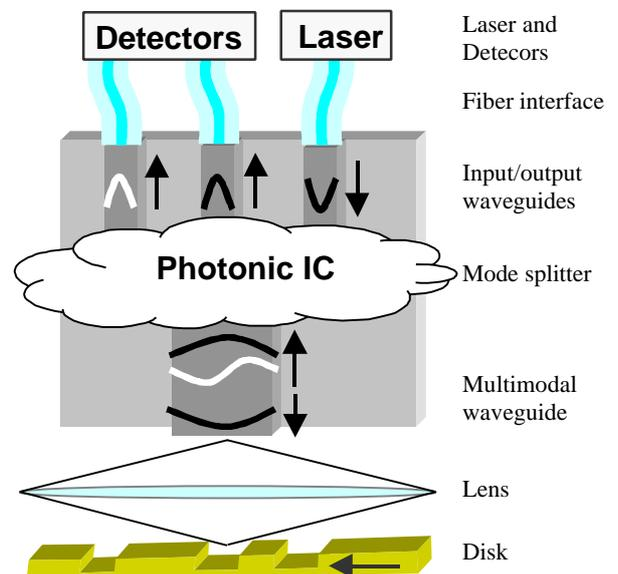
Figure 1: Schematic view of the PIC, waveguide and disk.
