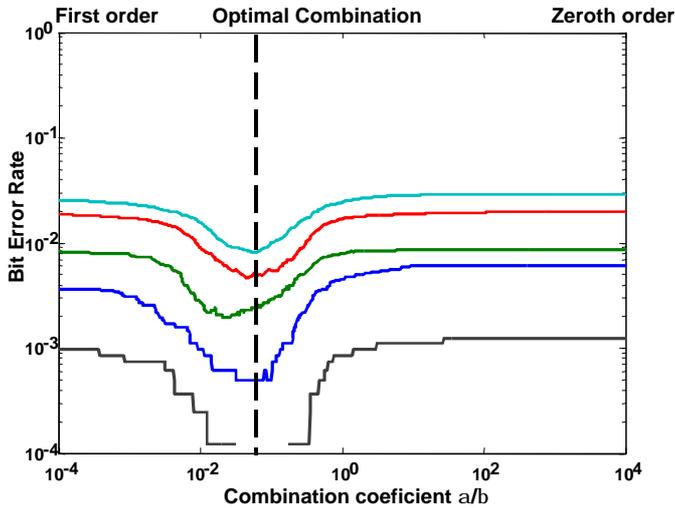
Figure 5: Bit error rates as a function of the linear combination of the two responses. The different curves denote different amount of noise.
