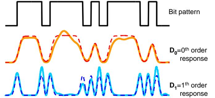
Figure 3: Bit pattern with zeroth and first order response.
