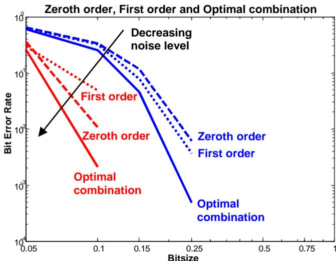
Figure 6: Bit error rate as a function of bit size (in  $\lambda/\text{NA}$ ) units
