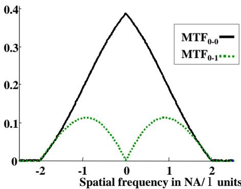
Figure 2: Modulation transfer function for zeroth and first order response.
