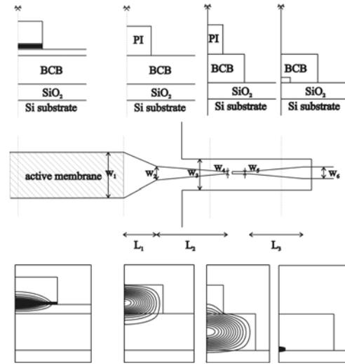
Fig. 4. BCB bonding coupling scheme - layout and mode transformation
