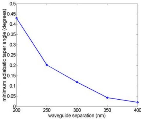
Fig. 3. Minimum adiabatic taper angle versus waveguide separation for SOG bonding coupling scheme
