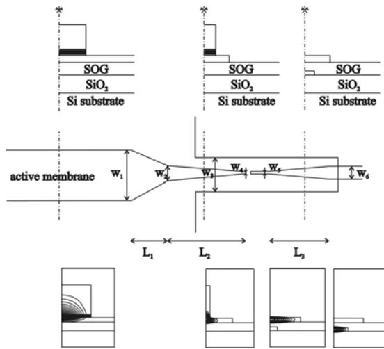
Fig. 2. SOG bonding coupling scheme – layout and mode transformation
