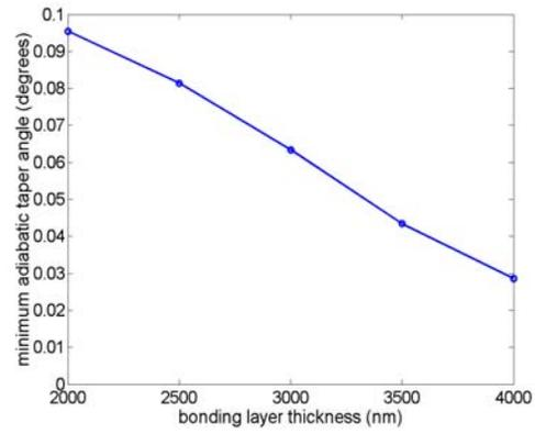
Fig. 5. Minimum adiabatic taper angle versus bonding layer thickness for BCB bonding coupling scheme
