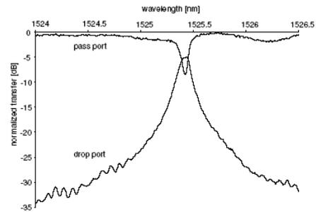
Fig. 6. Transmission to the pass and drop output ports of the ring resonator in Fig. 3c
