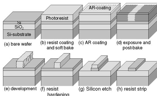
Fig. 1. The fabrication process for nanophotonic waveguide structures in SOI
