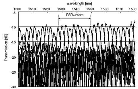
Fig. 4. Transmission to the 8 output channels of the AWG in Fig. 3a
