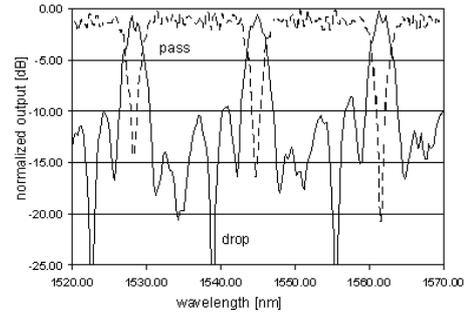
Fig. 5. Transmission to the pass and drop output ports of the CMZ in Fig. 2b
