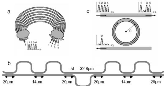
Fig. 2. Schematics of (a) an arrayed waveguide grating (b) a measured 5-stage cascaded Mach-Zehnder (c) a ring resonator
