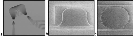
Fig. 3. SEM pictures of (a) an arrayed waveguide grating (b) one stage of a cascaded Mach-Zehnder with  $10 \mu\text{m}$  bend radius (c) a ring resonator with  $8 \mu\text{m}$  radius
