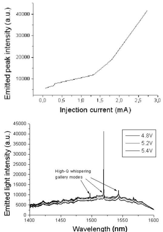
**Figure 3** PI-curve and emission spectrum of a membrane microdisk laser (diameter=8μm)
