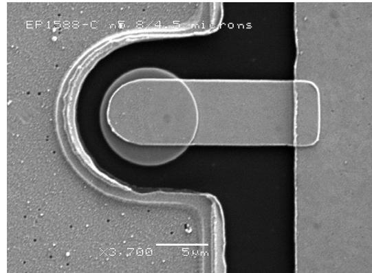
**Figure 2** SEM picture of a membrane microdisk laser
