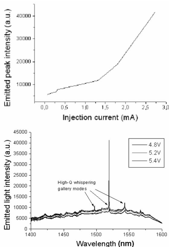
Fig. 3. Measurement results of an electrically injected membrane microdisk laser.
