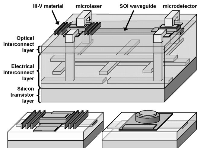
Fig. 1. Top: general layout of an SOI-based optical interconnect on CMOS. Bottom: two possible candidates for the membrane microlaser. Left: DBR-microlaser. Right: microdisk laser.
