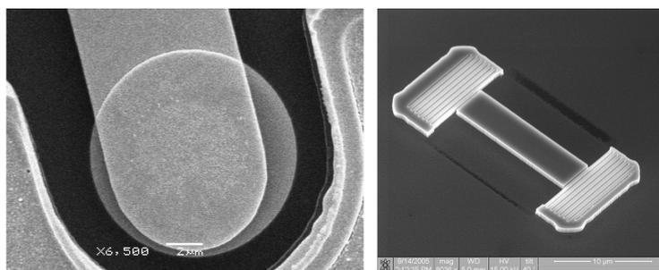
Fig. 2. SEM pictures of a fully processed microdisk laser (top) and an unfinished membrane DBR-microlaser (bottom).
