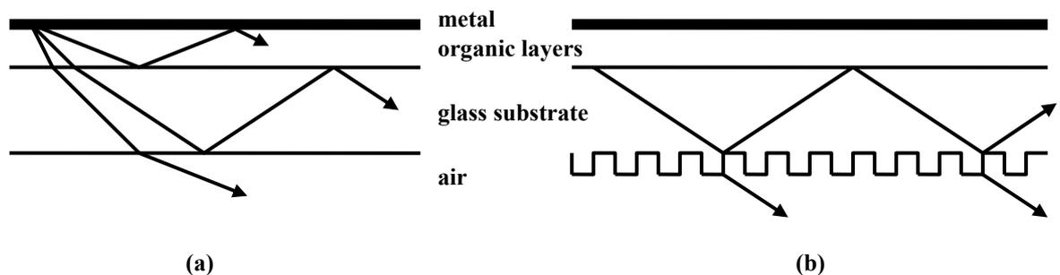
Figure 1. Extraction of light which is trapped for a planar structure.
