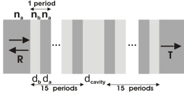
Figure 2: Two Bragg mirrors encapsulate a cavity. ( $\lambda_{resonance} = 1.56\mu m$ )
