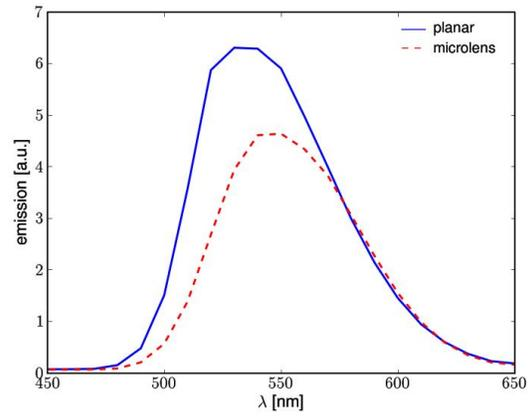
(b) RC<sup>2</sup>LED, absolute measurements, without and with microlenses
