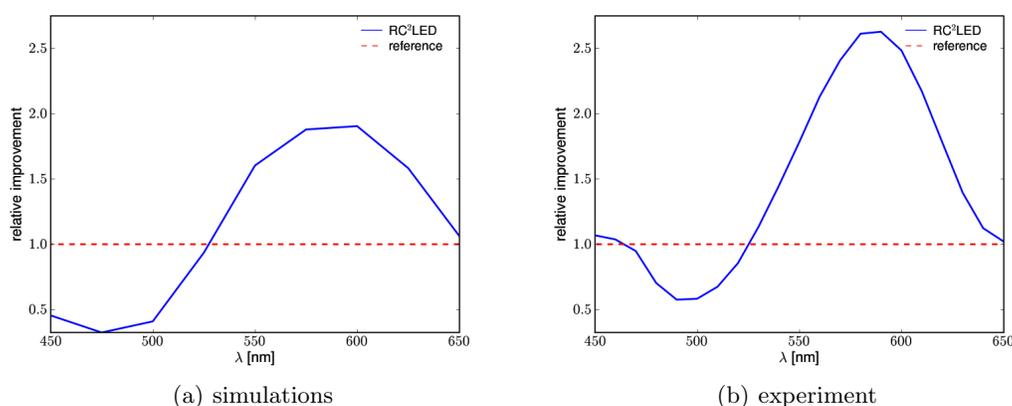
**Figure 5.** Relative improvement of the RC<sup>2</sup>LED and the reference OLED
