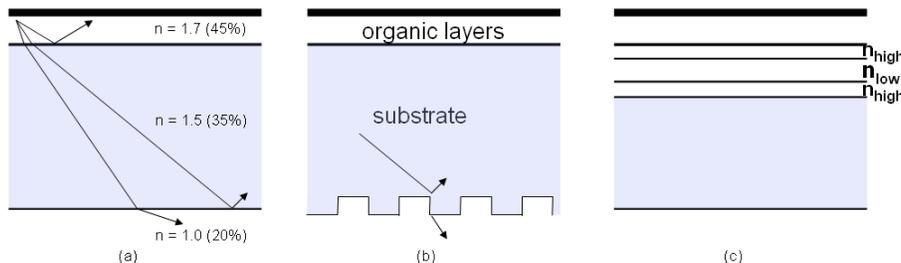
**Figure 1.** (a) Light extraction is limited by total internal reflection. The percentages are an estimation of the amount of light in each layer. (b) The grating at the interface between substrate and air. (c) An RC<sup>2</sup>LED is an OLED fabricated on top of a cavity. The cavity is made from a low refractive index material sandwiched between 2 high refractive index layers.
