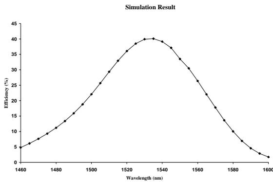
**Fig. 2:** Simulation of coupling efficiency as a function of wavelength of a gold grating coupler with the following grating parameters: period =  $610 \text{ nm}$ , filling factor =  $50 \%$ , height =  $20 \text{ nm}$ .
