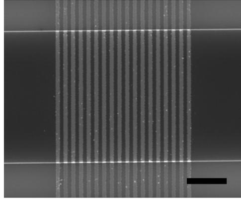
**Fig. 4:** Top view of the fabricated gold grating coupler on top of an SOI waveguide. Reference bar length =  $3 \mu\text{m}$ .
