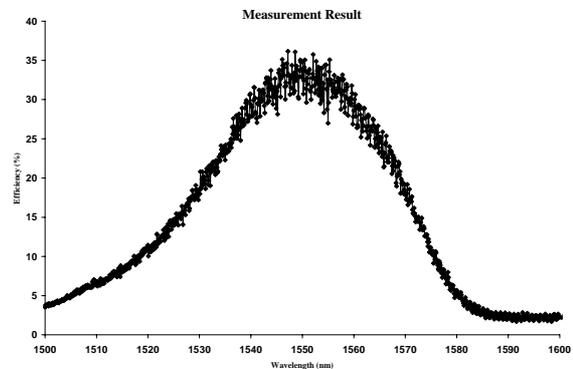
**Fig. 5:** Experimentally obtained coupling efficiency of a gold grating coupler on top of an SOI waveguide as a function of wavelength.
