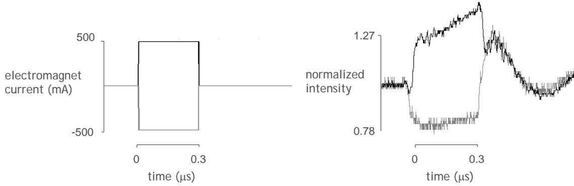
Figure 2: (left) Time evolution of the injected (pulsed) current in the electromagnet. (right) Corresponding (normalized) intensity emitted by the optical isolator at a bias current of 140mA (= above threshold).
