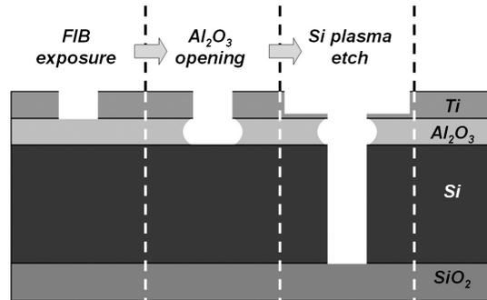
Figure 1. Schematic overview of the three-step process flow. In the first step  $\text{Al}_2\text{O}_3$  acts as etch stop layer and protects the silicon, in the final step  $\text{Al}_2\text{O}_3$  is again etched slowly and acts as hard mask.
