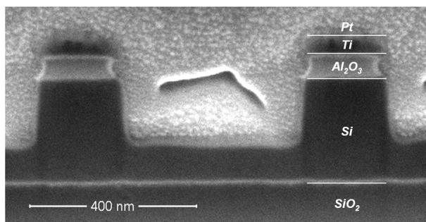
Figure 3. Cross-section micrograph of fabricated 400 nm wide and 150 nm deep trenches in the top 220 nm silicon layer of a silicon-on-insulator. Some Ti is still visible on top of the  $\text{Al}_2\text{O}_3$ .
