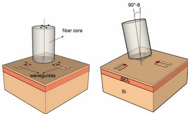
Figure 1. Polarization diversity using focusing grating couplers. (Left) Vertical fiber. (Right) Near vertical fiber in order to avoid second order reflections.
