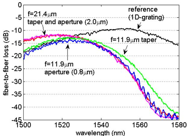
Figure 4. Fiber-to-fiber transmission for both configurations (short taper and shallow aperture) and different focal distances.
