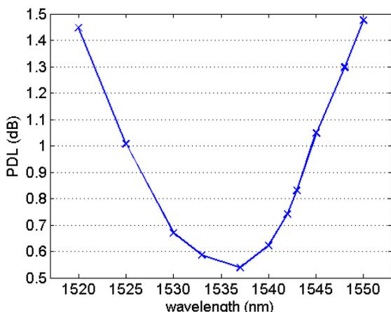
Figure 5. Measurement of the Polarization Dependent Loss.
