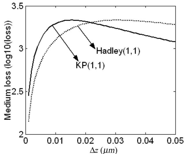
Fig. 3. Medium loss of WA beam propagation using CJI based on Hadley(1,1) (dotted curve) and  $KP(1,1)$  approximant (solid curve).
