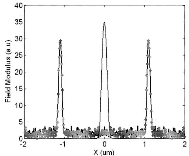
Fig. 4. Input beam at  $z = 0$  (solid curve that peaks in center) and output beam at  $z = 21 \mu\text{m}$  in a 2D Y-branch rib waveguide calculated by WA-BPM based on  $KP(1,1)$  (solid curve that peaks on left and right) and Hadley(1,1) (circles).
