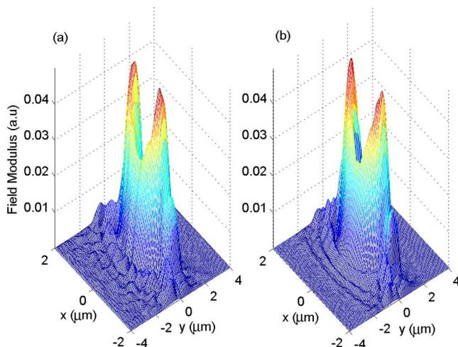
Fig. 5. (Color online) Magnitude of TE fundamental mode after propagating  $3 \mu\text{m}$  in a 3D Y-branch rib waveguide calculated by WA-BPM based on (a)  $KP(1,1)$  and (b) Hadley(1,1).
