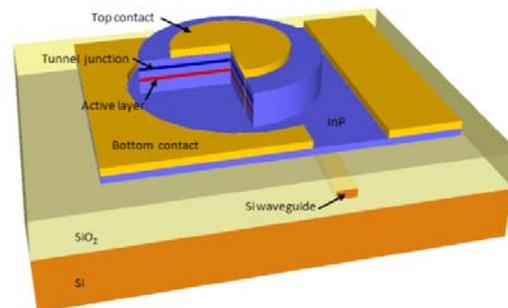
**Fig. 3: Microdisk source schematic**
