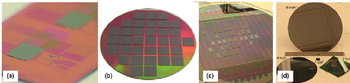
**Fig. 2: (a) BCB-bonded InP dies on SOI (from [1]) (b) BCB-bonded InP dies on IBM CMOS (from [2]) (c) InP dies on SOI through molecular bonding (see [3, 4]) (d) Direct bonded InP-wafers on SOI (from [5, 6])**
