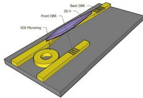
Figure 6. The schematic of adiabatically tapered heterogeneously integrated III-V/Si for a single mode laser.
