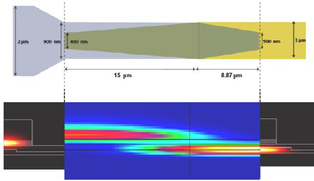
Figure 5. a mode transfer structure with optimize taper length.
