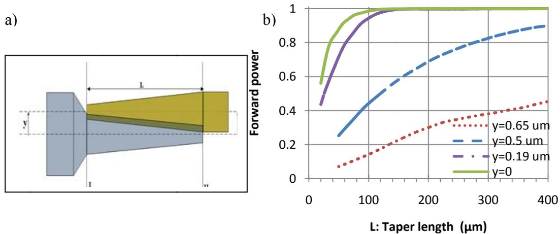
Figure 4. a) the layout for the lateral misalignment of  $y$  b) the forward power of fundamental mode versus the taper length of  $L$  for different values of  $y$  and BCB thickness 80nm.
