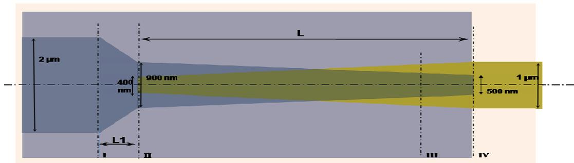
Figure 2. The layout of adiabatic tapered III-V/silicon for the first design
