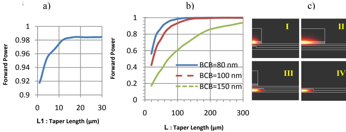
Figure 3. Forward power for the fundamental mode for various taper length a) first taper b) second taper for different value of BCB thickness c) an example for fundamental mode profile in four different cross-sections are shown in figure 2.
