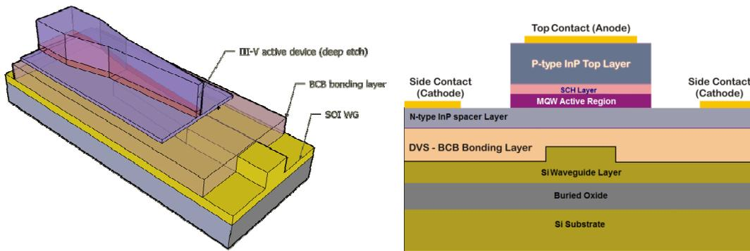
Figure 1. The schematic of adiabatic tapered III-V/silicon laser and cross-section
