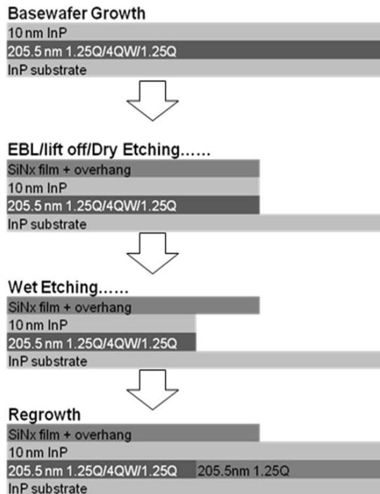
Figure 10. Fabrication process flow
