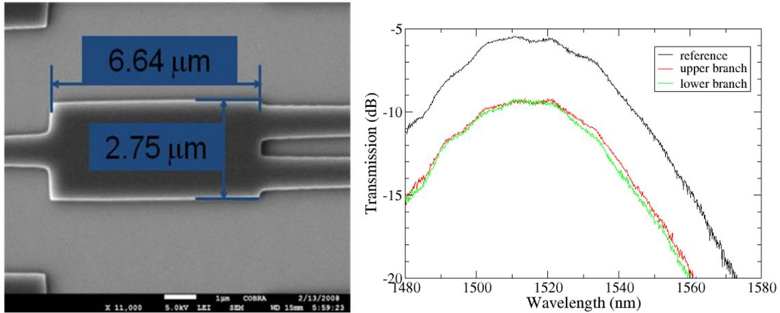
Fig.5: left – SEM image of a fabricated MMI ; right – transmission through both output branches, together with the reference, connected to two grating couplers.
