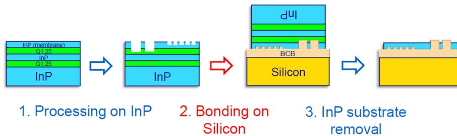
Figure 2: IMOS fabrication scheme
