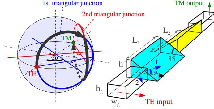
Figure 7: Schematic of the polarization converter design and Poincaré sphere diagram of the polarization conversion.
