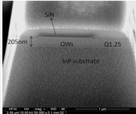
Figure 12. Cross section made by FIB
