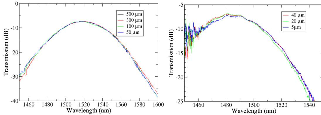
Fig. 4 Left: Transmission through 400 nm wide wires of different lengths, connected to two grating couplers.
