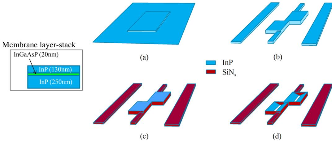
Figure 9: Fabrication process design for the PC
