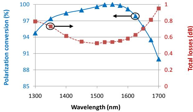
Figure 8: Spectral behaviour of the proposed PC design optimized for  $\lambda = 1.55 \mu\text{m}$
