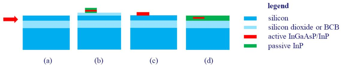
Figure 1: Schematics of four different ways to generate light in a photonic layer on top of a silicon IC
