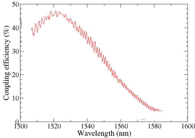
Fig. 3: Coupling efficiency for the grating coupler.
