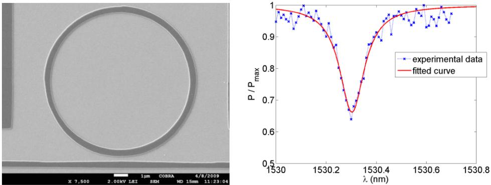
Fig. 6: Left-SEM photograph of the ring resonator with 7 μm radius. Right-transmission spectrum at the resonance peak.
