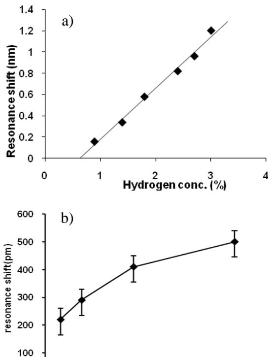
Fig 2a) measured response from the hydrogen sensor, b) measured response from the ethanol sensor
