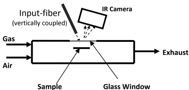
Fig 1 measurement setup
