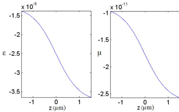
**Figure 3.** The permittivity and permeability vary along the propagation direction according to a hyperbolic tangent function assumed in this paper.
