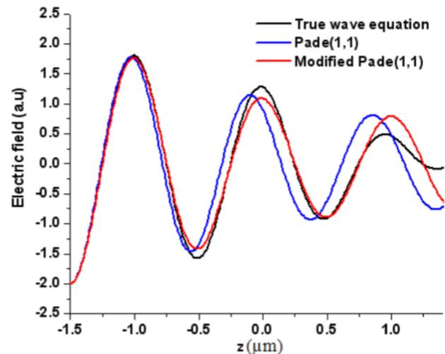
**Figure 4.** Propagation of electric wave in graded-index structure with positive index profile changing according to hyperbolic tangent function.
