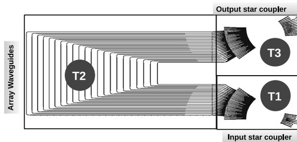
**Figure 4:** Diagram of Simulation approach for a AWG.
