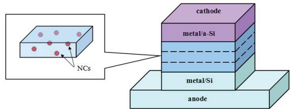
Figure 1. Schematics of the models for the light source and the NCs.
