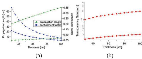
Figure 2. Propagation length, confinement factor (a) and transparency gain (b) for different total thickness in the NC light sources on Si (solid lines) and in the NC light sources for SPPs (dashed lines).
