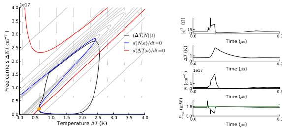
Figure 4: A temporary increase of  $P_{in} = 1.8$  mW at  $\delta\lambda = -16$  pm to 2.9 mW, during 2 ns, triggers an excitation. Although for this input power no limit cycle is present, the excitation can be seen as a reminiscent of the nearby limit cycle from Fig. 3.
