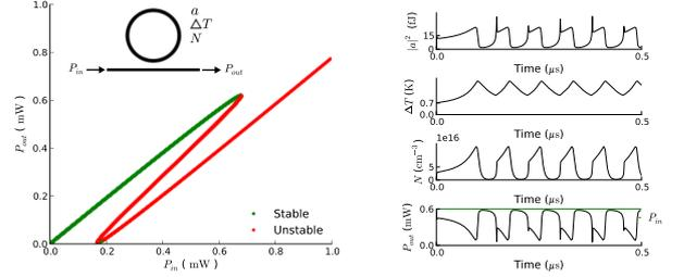
Figure 1: For detuning  $\lambda - \lambda_r = 62$  nm,  $P_{out}(P_{in})$  is bistable (left side figure), for  $P_{in}$  higher then  $\approx 190 \mu\text{W}$  the lower  $P_{out}$ -branch gets unstable, which is an indication of self-pulsation. For  $P_{in} = 600 \mu\text{W}$  and  $(a, \Delta T, N)(t=0) = (0, 0.7, 0)$  this gives the self-pulsation timetrace on the right.
