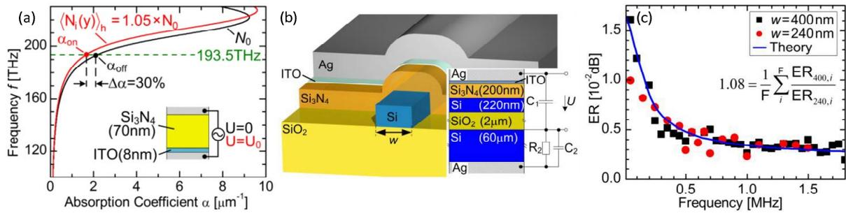
Figure 3. The dispersion relation (DR) of SPP at Ag / ITO / Si<sub>3</sub>N<sub>4</sub> / Ag structure and the schematic of the device fabricated for proof-of-principle experiments: (a) DR of SPP at Ag / ITO (8 nm) / Si<sub>3</sub>N<sub>4</sub> (70 nm) / Ag for 10 V<sub>pp</sub> voltage on and off states, (b) The schematic of the fabricated devices and (c) the measured extinction ratio.
